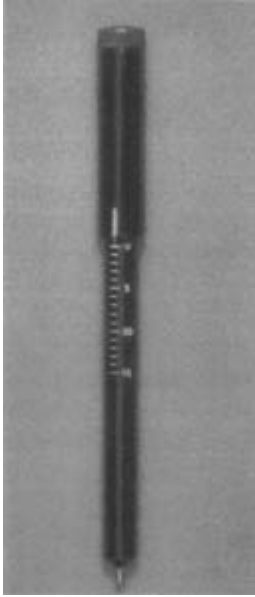
Figure 2 A dermographometer, a pen-like instrument containing a spring. The markings can be calibrated, with the settings of this instrument being 0 = 20.4 g/mm 2 , 5 = 59.9 g/mm 2 , 10 = 99.4 g/mm 2 , and 15 = 1144 g/mm 2 .
