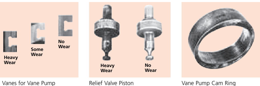
Figure 1. Typical Examples of Wear Due to Contamination
