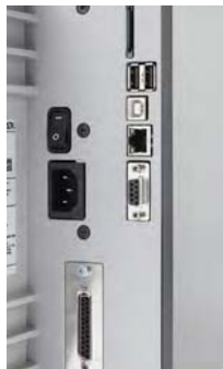
Various connectivity options on the BradyPrinter i7100 Industrial Label Printer
