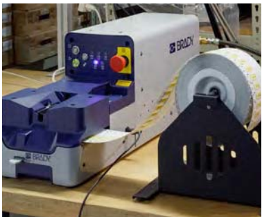
Feed printed PermaSleeve roll into the BSP45 Applicator
