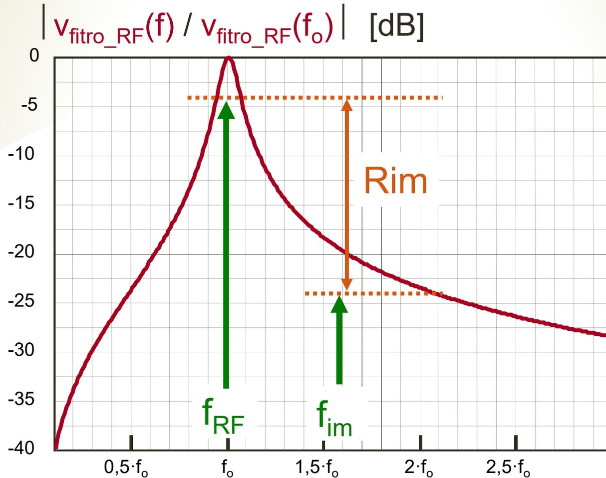
$$R_{Im} = \frac{A_O}{A_{FI}} = \sqrt{1 + Q_C^2 \left( \frac{f_0}{f_i} - \frac{f_i}{f_0} \right)^2}$$
