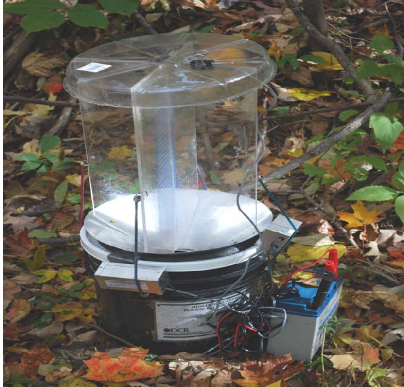
Figure 17. Ultraviolet light trap used for invertebrate sampling at Powell Mountain Karst Preserve, Wise County, Virginia
