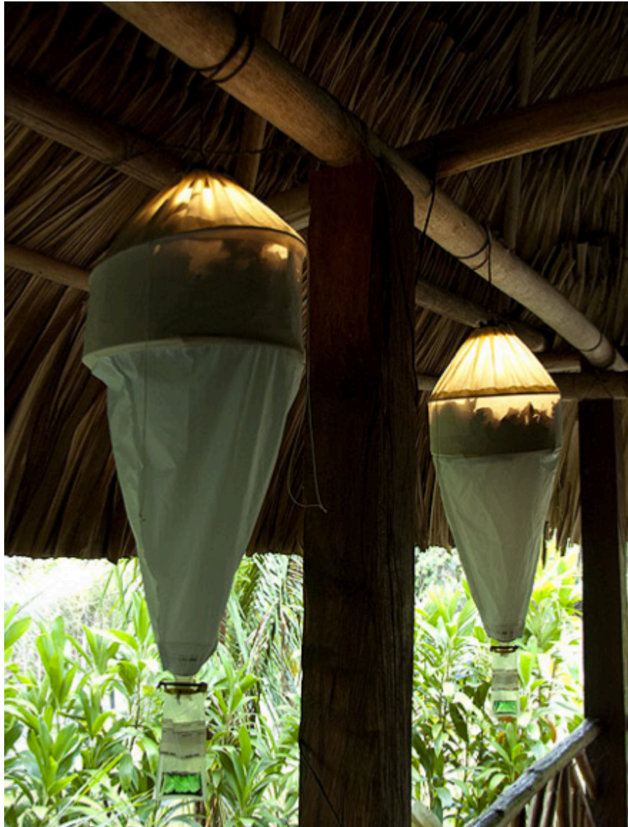
Figure 4. Portable Berlese funnels were used to extract small invertebrates from leaf litter samples taken near cave entrances. Photo © Geoff Hoese/SEI.
