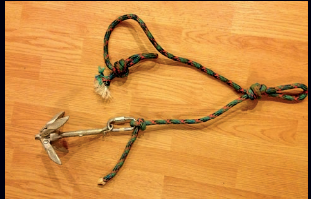
Page 28: A portion of the rigging used by 2 stranded cavers in Ophir Cave, Montana. The kayak anchor was placed among rocks and the Walmart rope was knotted for handholds. No backup knot was used at the rope/anchor interface. The frayed end was cut by rescuers. Photo: Duncan Adams.
