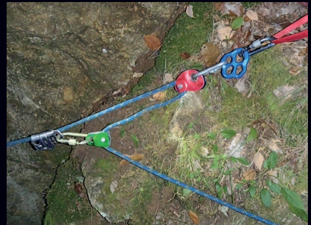
Page 34: An improvised 3:1 haul system used to extricate a caver from War Eagle Cave, Alabama. All of the gear came from the pack and personal vertical system of just one caver in the group. Photo: Glen Kuehner.
