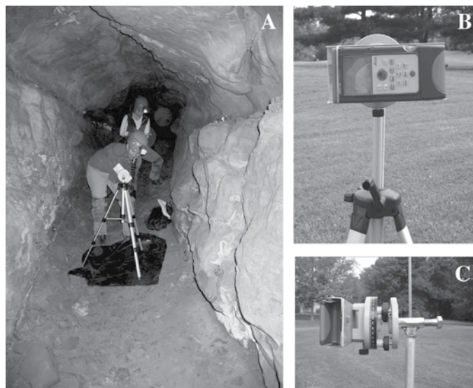
Figure 4. Equipment used for precise radial surveys. Device shown in use within Scott Hollow Cave (A). Disto laser measurement device by Leica is mounted on a tripod using a modified transit head (B, C). Arrangement allows both for leveling of device, and rotation through full 360 degrees of measurement.
