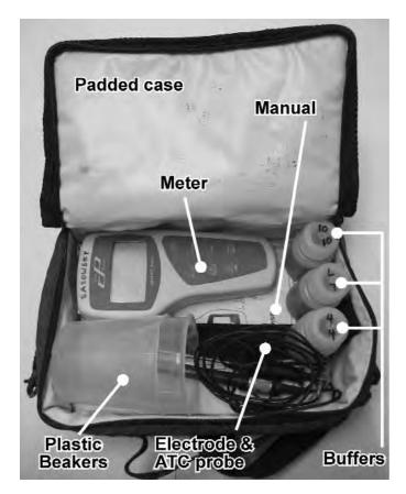
Figure 2. Example of a kit for field pH measurement in karst settings.
