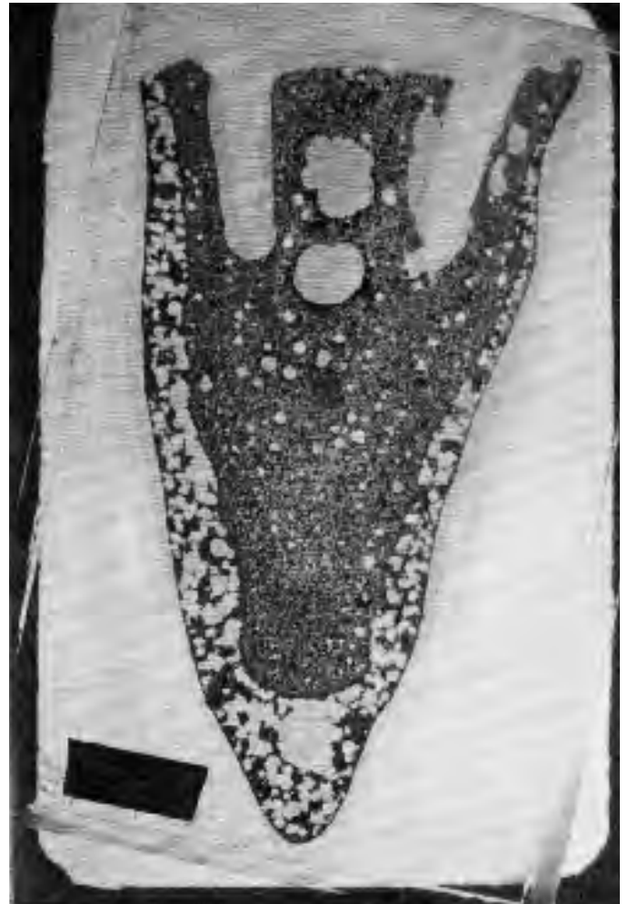
Figure 7. The HA1 shark tooth stalactite thin section. Eight linings are visible with magnification. The light voids are vesicles. The sample is 66 mm long. Photo by M. Palmer.
