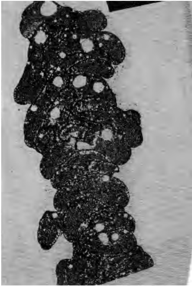
Figure 13. A thin section of lava stalagmite HA4. The light voids are vesicles. Sample is 56 mm long. Photo by M. Palmer.
