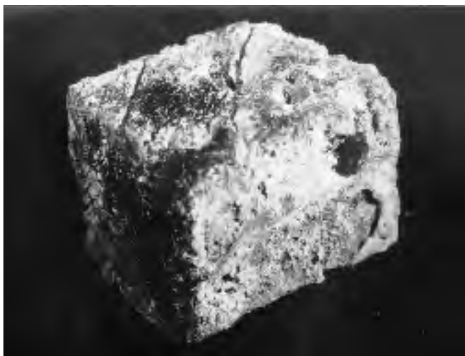
Figure 3. A remnant of thermal fluorite with visible traces of corrosion.
