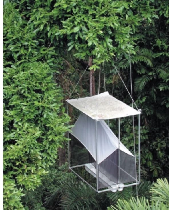
Fig. 70. Composite Malaise-Flight Interception trap hanging in the mid-canopy (photo Michael Cermak).
