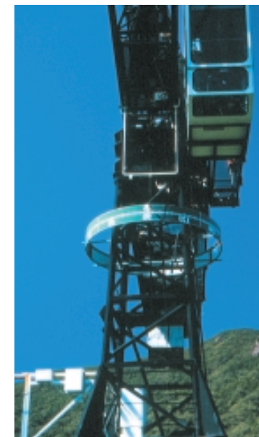
Fig. 68. The crane has a positioning system designed to allow researchers to accurately and quickly find sites within the canopy (photo Michael Cermak).
