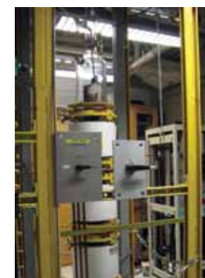
Another view of the renovated 6-inch glass distillation column in our Unit Operations Lab
