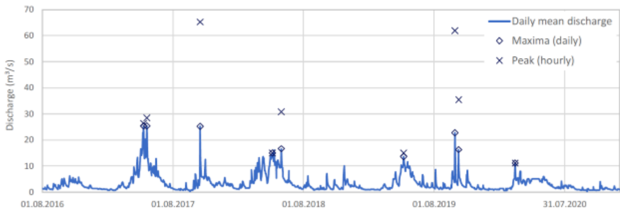
Figure 5.3.3.3.1.2. Observed peak and peak discharge calculated from daily mean data for Bakhvi 3 peaks
