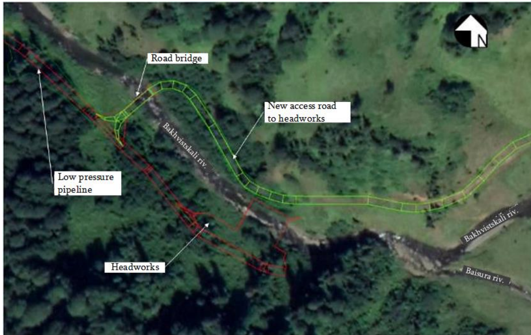
Figure 3.1.4.2. Layout scheme of headworks
