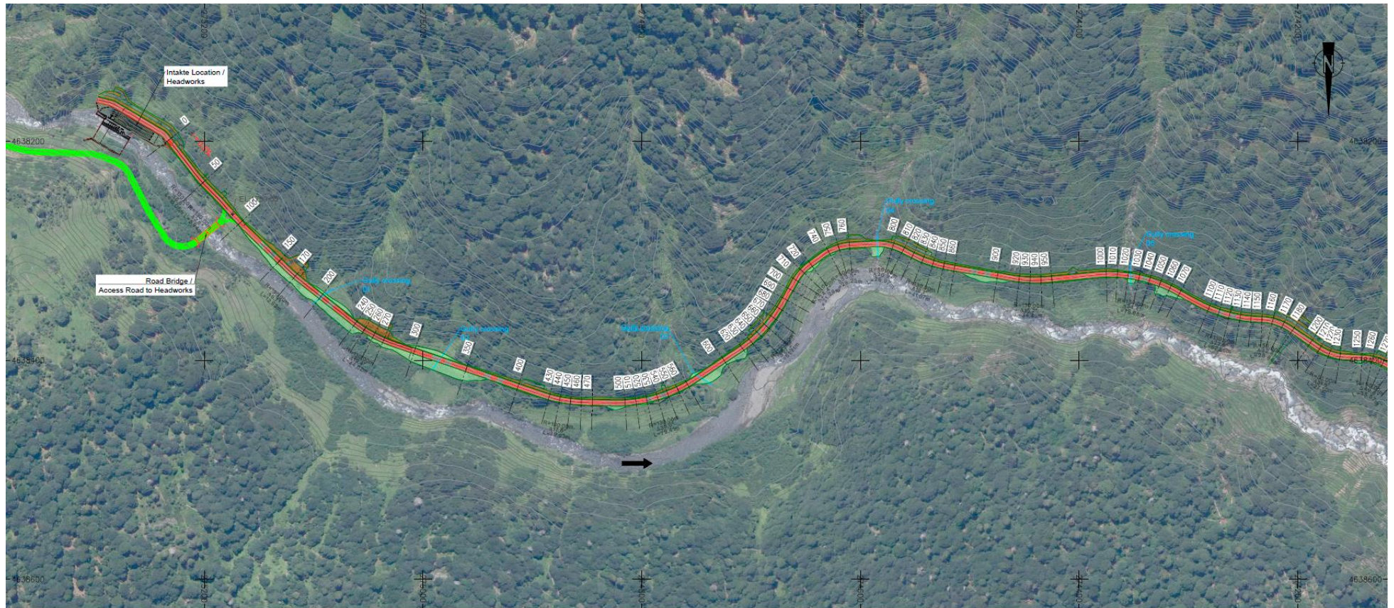
Figure 4.1.2.1. Scheme of penstock (3 parts)
