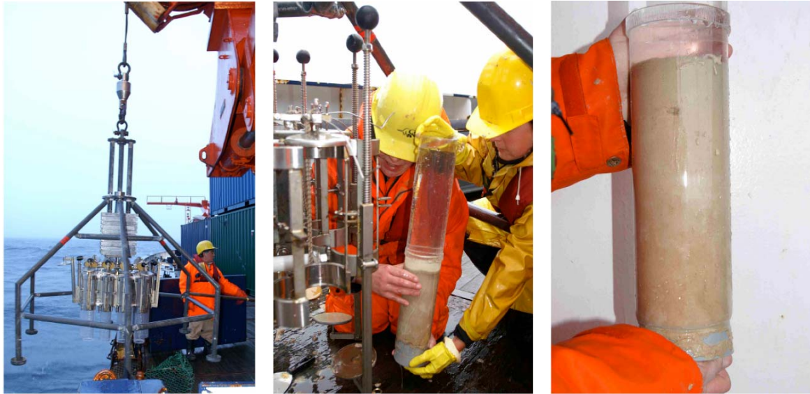
Fig. 15.4: (from left to right): Deployment of the Multicorer from board Polarstern; removal of filled cores on deck; successful sediment core from station PS 71/13-12, 2963 meters depth
