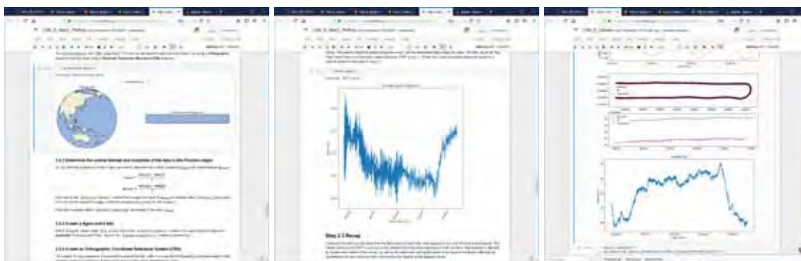
Figure 53-6. In the first assignment, implemented through a set of Python Notebooks, students are presented with data collected in the West Pacific (left), they proceed by integrating the raw echosounder observables (middle) with the positioning, motion and tide data to derive georeferenced depth data (right).
