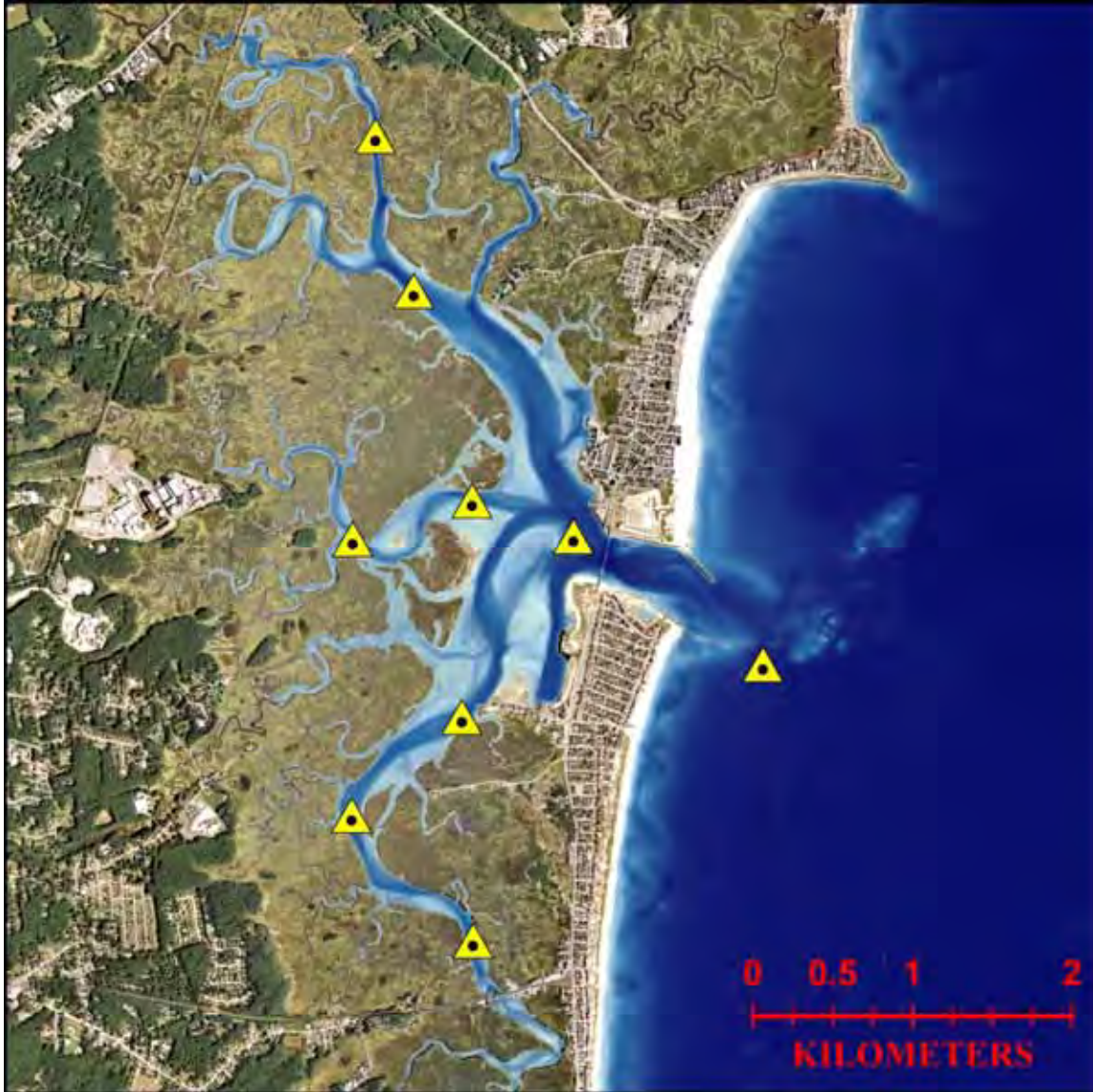
Figure 33-1. Map of Hampton Harbor showing the location of instruments deployed for 30 days in the fall of 2017 to measure wave, currents, temperature, salinity, and optical backscatter. Data from these instruments will be used to verify the hydrodynamic model and set the proper bottom boundary condition for the model.
