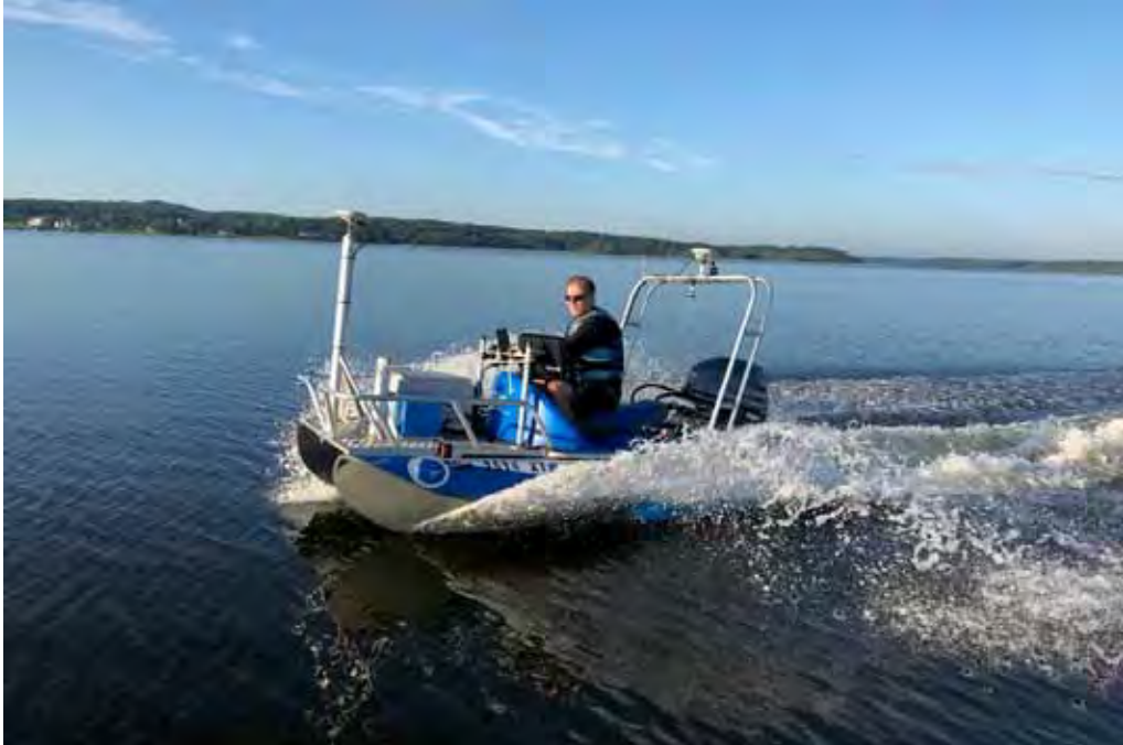
Figure I-12. The JHC Zego Boat, a highly maneuverable and stable twin-hulled catamaran that is being outfitted into a state-of-the-art shallow water survey vessel with MBES, SBES, and ADCP capabilities.
