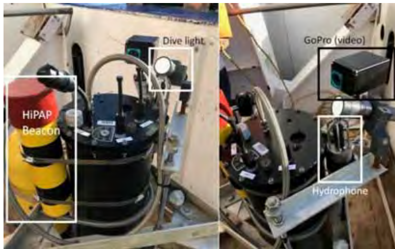
Figure 39-1. The bubble generator and auxiliary equipment employed during bubble generator deployment operations: positioning beacon, video camera/dive light, and hydrophone.
