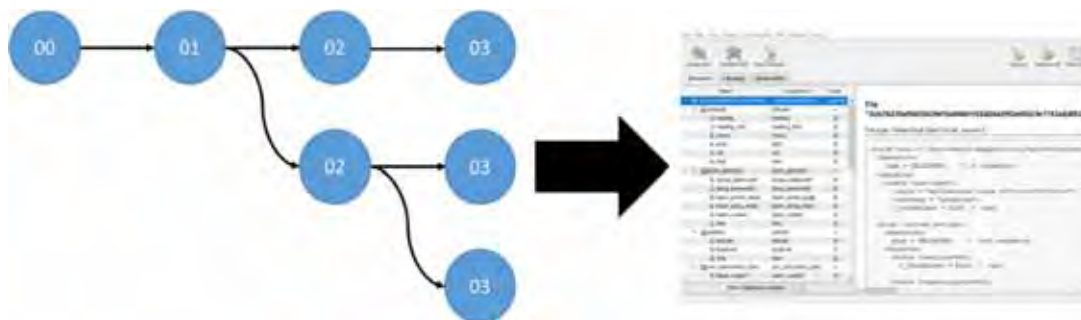
Figure 22-4. The processing workflow for OpenBST follows a directed acyclic graph (DAG) which leverages the NetCDF convention's self-descriptive and metadata coupling abilities to efficiently move through the backscatter processing workflow. On the left, the DAG diagram shows the results of a processing operation in the blue circle. On the right, a visualization of the sonar data in the NetCDF file obtained using NASA GISS' Panoply, a free software for netCDF file visualization.
