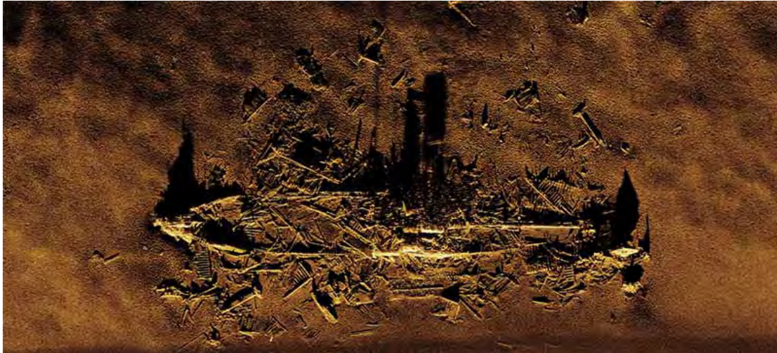
Figure 4-3. Synthetic aperture sonar image collected over a shipwreck site off of Virginia using the KATFISH towed SAS system.
