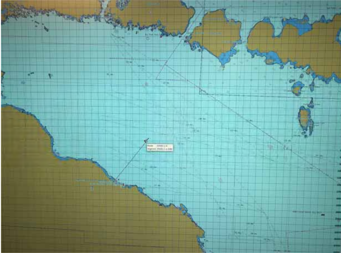
Figure 11-3. ASV-BEN, conducting test of sustainable telemetry range with the Kongsberg Marine Broadband Radio telemetry system. Here the ASV is some 20 km from the operating station, approaching the center of Lake Huron. This range resulted from exceptionally favorable conditions. More typical maximum ranges were 14-16 km.
