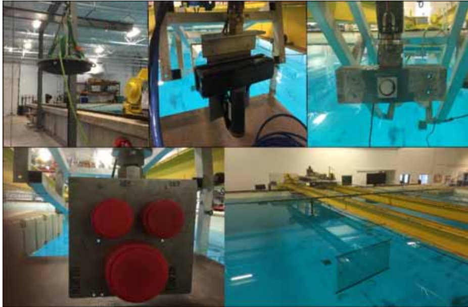
Figure 1.1. Tests in the acoustic tank in 2019. Top Left: MSI LF CBT; Top Center: Reson T50-P; Top Right: Custom-built transducer; Bottom Left: Simrad split-beam echosounders; Bottom Right: Standard chain target.
