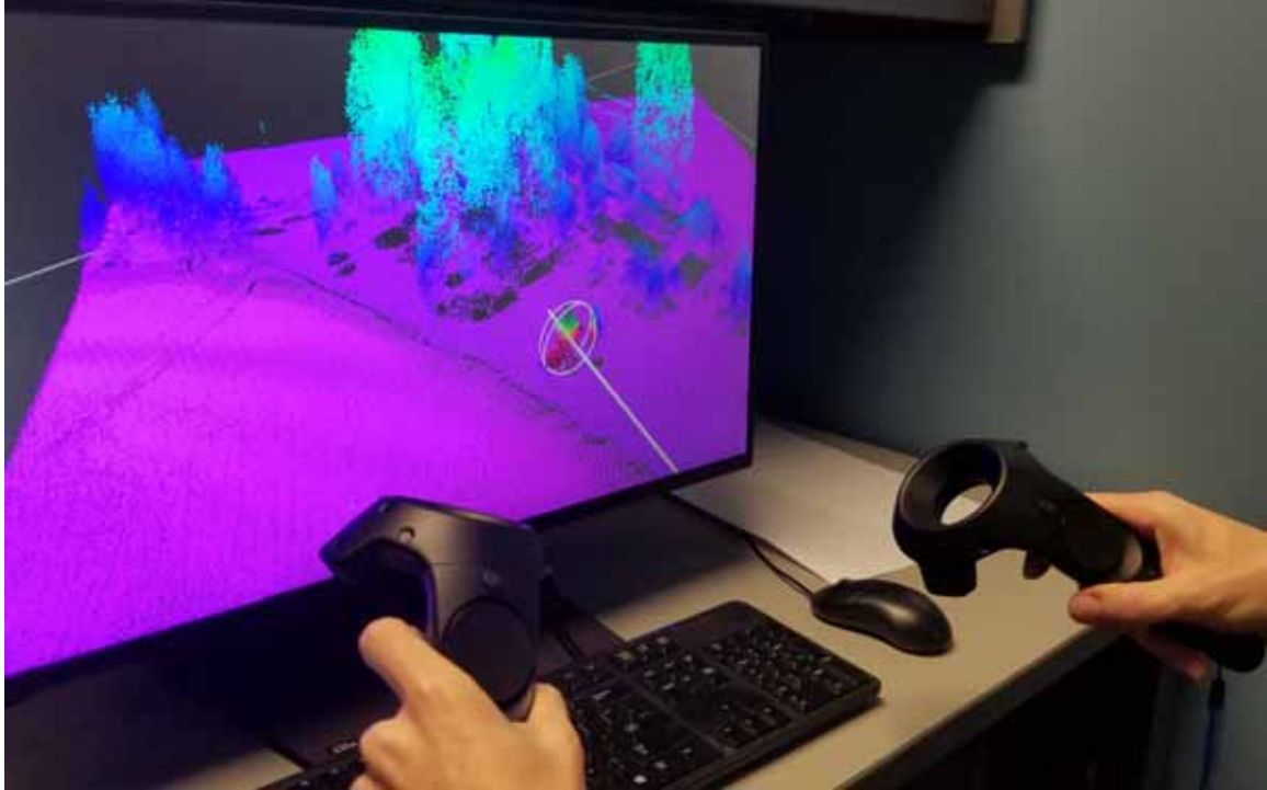
Figure 39-2. Editing coastal LIDAR point clouds with the latest version of our desktop editor, which uses a 3D monitor and 6DOF handheld controllers.
