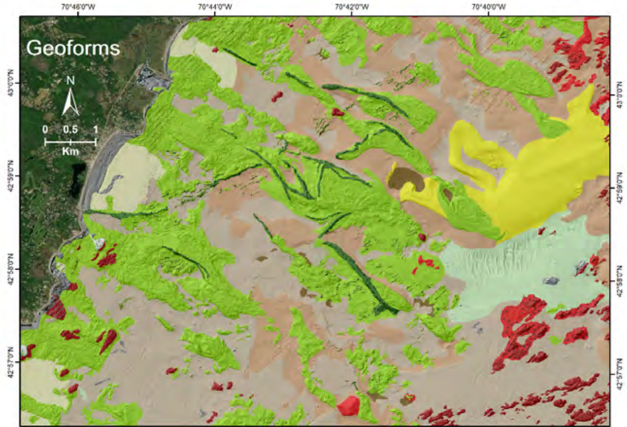
Figure 21-1. Surficial geology map of the nearshore continental shelf landward of the Isles of Shoals, NH showing the major geofoms. The seafloor is characterized by eroded glacial features (leaving behind megaclast deposits) and seafloor plains. The BRESS landform analysis of the same area is shown in Figure 21-2. Marine-modified glacial features are shown in green, marine formed features in yellow, seafloor plains in beige, depressions in brown, bedrock outcrops in red, nearshore ramps in ivory, and bedform fields in mint green. Dark grey areas are unmapped.
