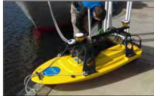
Figure I-15. Seafloor Systems' "Echoboat" (upper), Hydronalix "Emily Boat" (middle,) and Teledyne Oceansciences' "Z-Boat," small autonomous surface vessels used by the Center to develop autonomous command and control algorithms.
