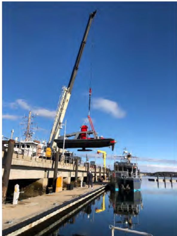
Figure I-16. iXblue DriX autonomous surface vehicle that has been delivered to the Center. On left is vehicle being lowered into the water in its Launch and Recovery System.
