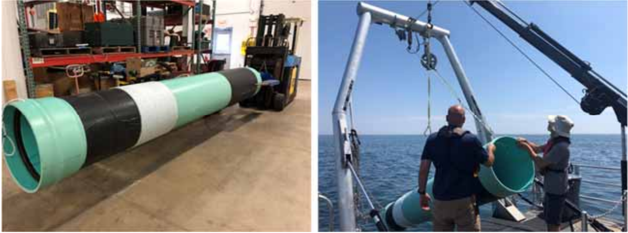
Figure 14-4. The pipe with a 'roughened' surface consisting of antiskid tape and a wrap of potwarp (left image), and the deployment of the pipe at sea using the R/V Gulf Surveyor.
