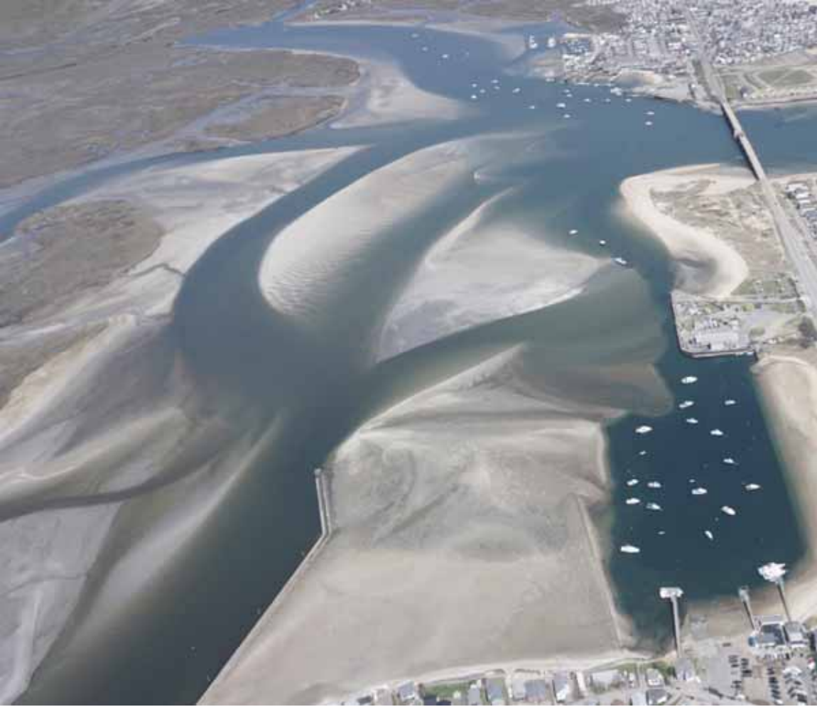
Figure 33-8. Aerial photograph of Hampton/Seabrook Harbor taken in 2017 showing the channel cuts across the middle ground (flood tidal delta) and infilling of the navigational channel leading to a large portion of New Hampshire's fishing fleet.
