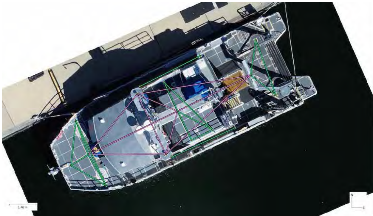
Figure 12-5. Orthomosaic of the R/V Gulf Surveyor corresponding to the point-cloud of Figure 12-3. Note the lines joining survey monuments (purple) and Secchi targets (green), which are measured in the orthomosaic to assess the technique.
