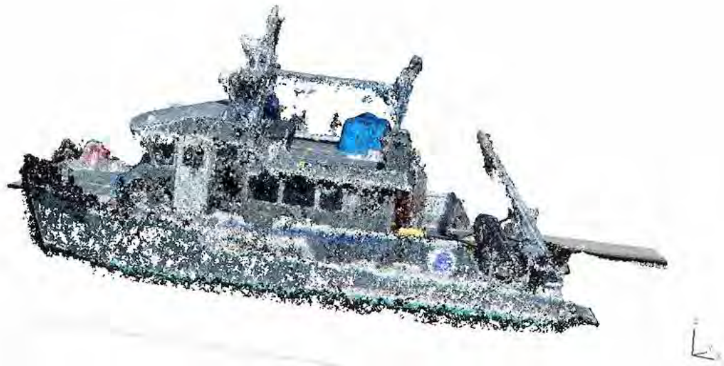
Figure 12-4. Point-cloud for the R/V Gulf Surveyor constructed using Structure from Motion (SfM) techniques applied to the drone photogrammetry survey at an altitude of 31m.
