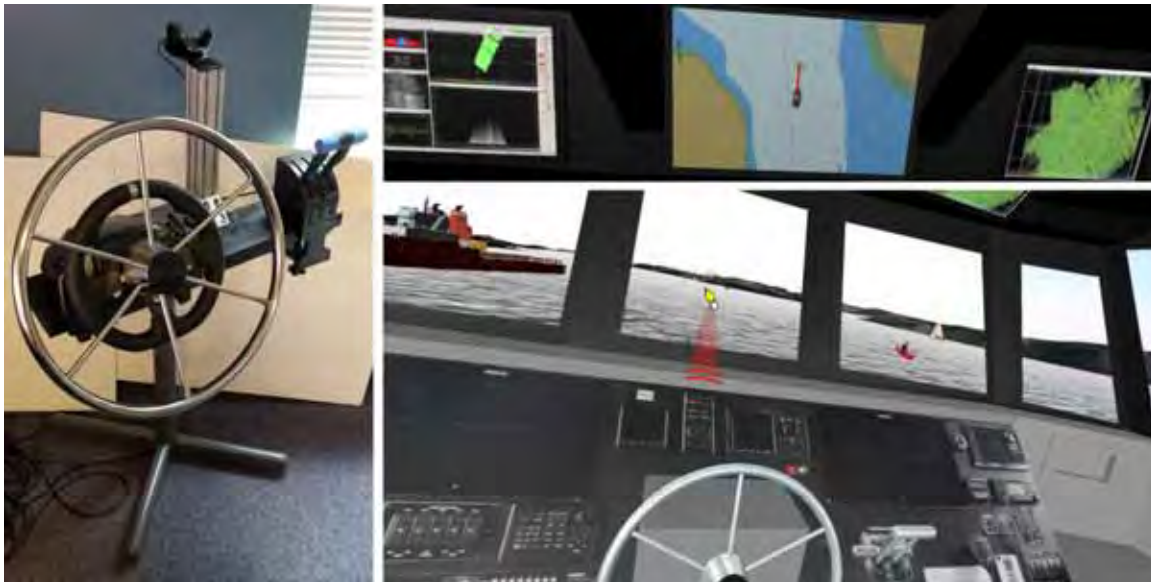
Figure 44-2. The virtual bridge and AR simulator. (left) The physical controls used to pilot the boat. (right below) View from the virtual bridge within the field-of-view study environment, showing ship traffic and AR trackline to next waypoint. (right above) The virtual ECDIS display above the bridge windows, showing a track-up OpenCPN chart with the same trackline and waypoint.
