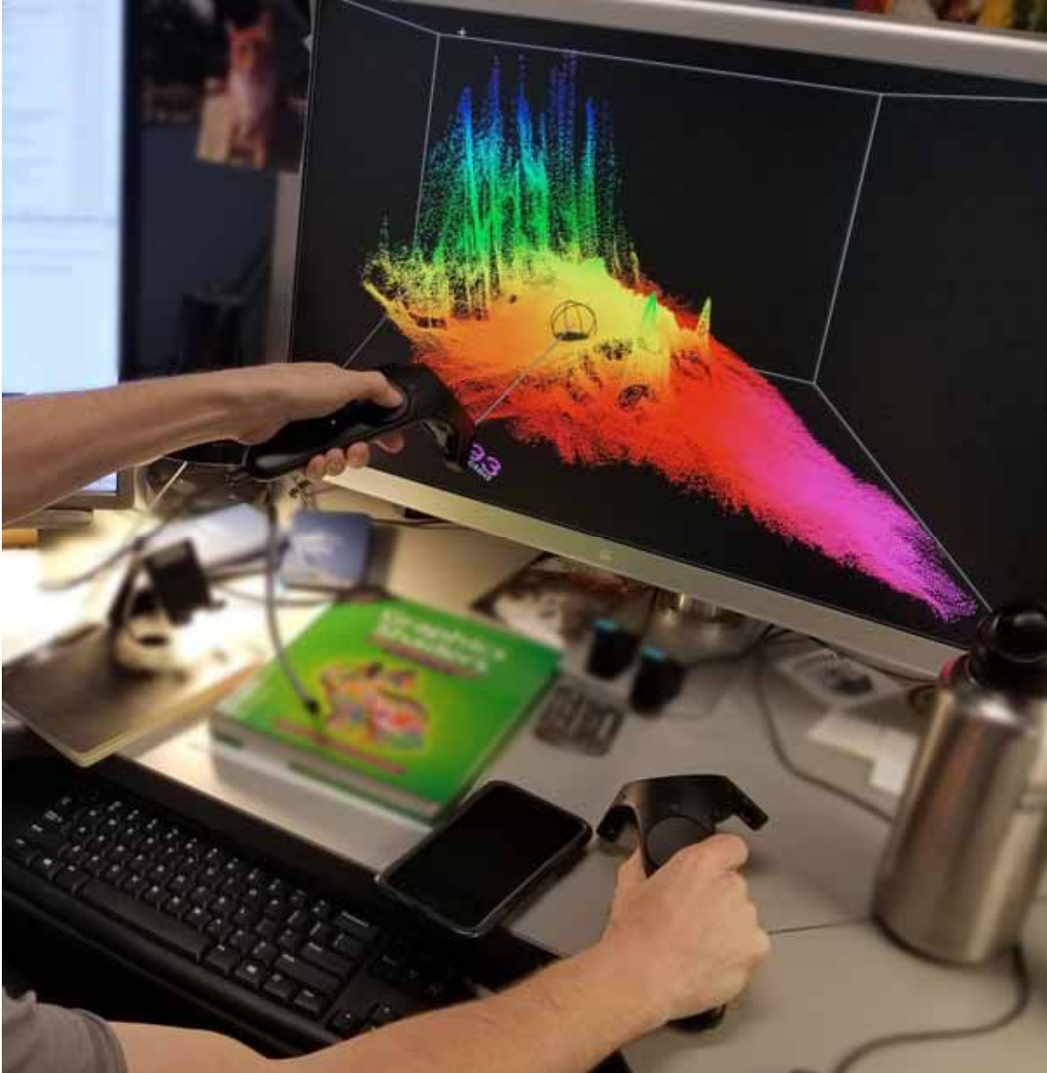
Figure 39-1. Our point cloud editor being used on a standard 2D desktop monitor, where the 6DOF handheld controllers can be used to “reach into the screen” and edit, manipulate, reposition, and scale data similar to the immersive mode.
