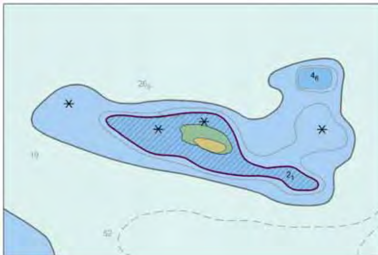
Figure 37-10. Depth area encoded in different units than the adjoining depth area and the delimited depth curve (i.e., fathoms vs meters).
