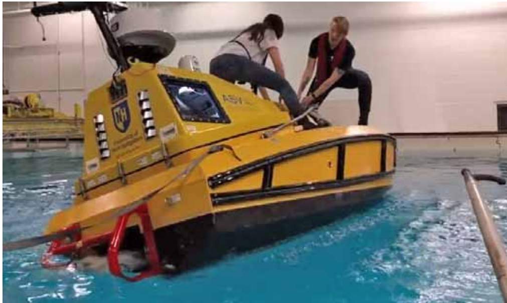
Figure I-6. Engineering test tank being used to test the IMU and multibeam on the BEN (Bathymetric Explorer and Navigator) ASV.
