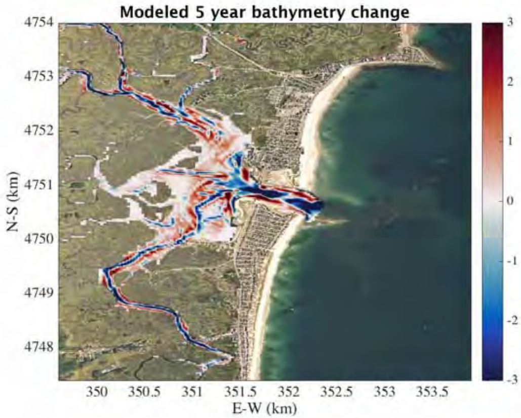
Figure 33-6. Bathymetric difference map from the five- year model run showing distribution of erosion and deposition.
