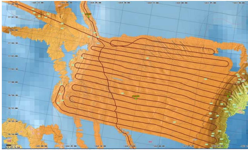
Figure 43 – overview of ice scour survey – note dune-like features to south
