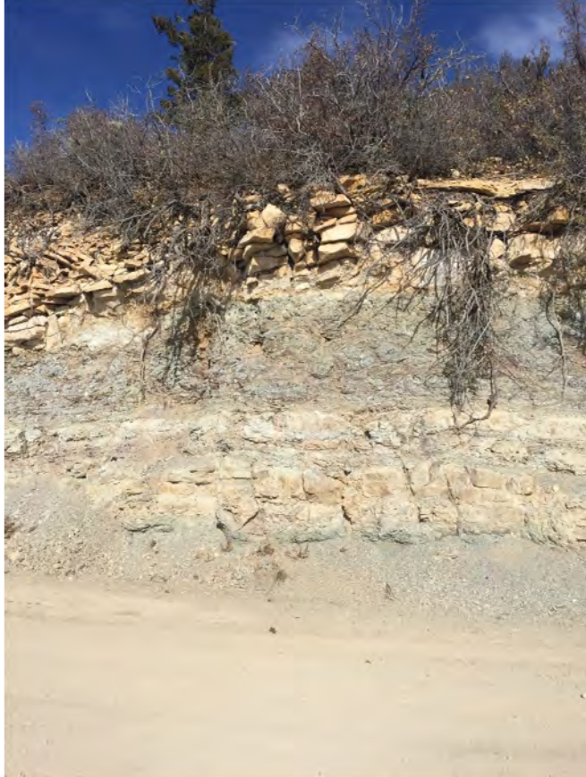
Interbedded shale and sandstone of Green River Formation, highly fractured and horizontally bedded, at Book Cliffs Ridge Road
