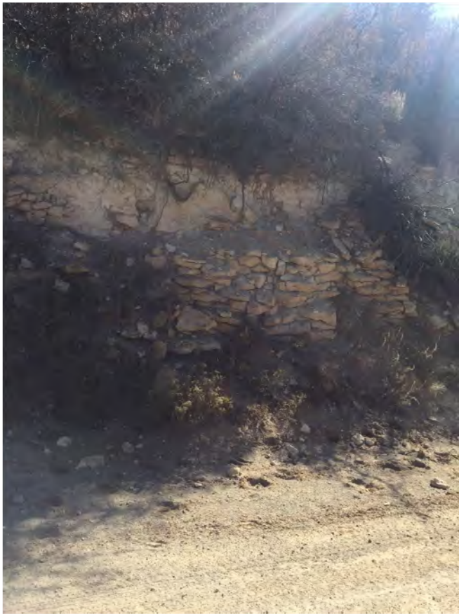
Highly fractured, highly jointed, down-dipping sandstone of Wasatch Formation observed at near Book Cliffs Ridge Road/East Canyon Road crest
