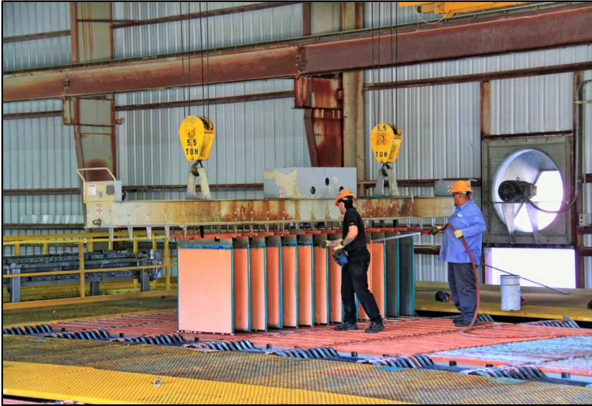
Figure 93. Pulling copper cathodes at electrowinning tank house at Carlota (photo from KGHM)
