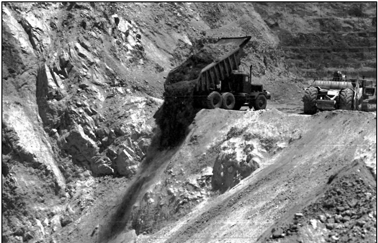
Figure 78. Haul truck dumping ore in a 65-foot by 100-foot glory hole caved block transfer in Thornton pit, circa 1950s (photo from Hardwick, 1963)
