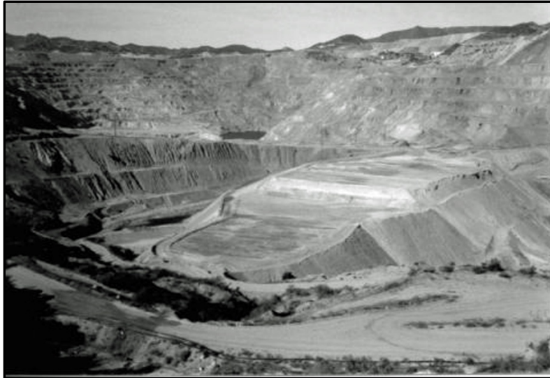
Figure 69. Tailings disposal in the inactive Copper Cities pit, circa 1990s (photo from Arizona Geological Survey)
