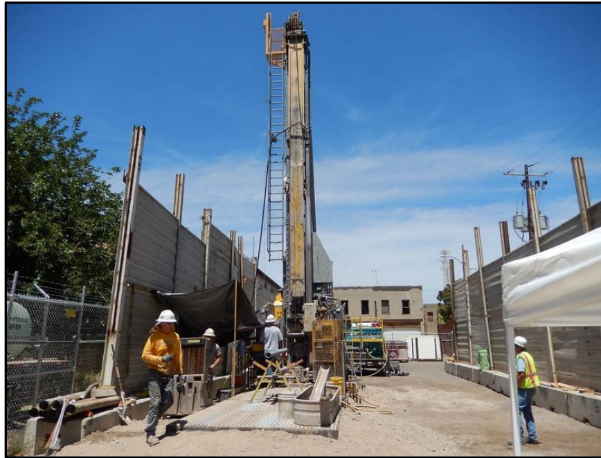
Figure 96. Diamond drilling in the parking lot adjacent to the Miami mayor and council building, circa 2014 (photo from Copper Fox Metals, Inc.)
