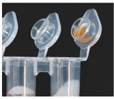
Streptavidin Bead Adherence to Tube Wall during Washes is Normal
