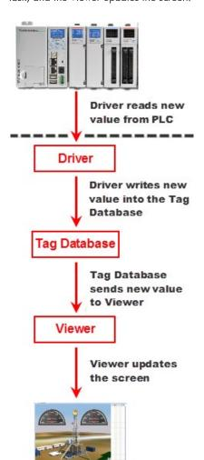
Note that the driver does not send new tag values directly to the Viewer. In addition, there is no pooling between tasks — the tag database receives the updated information and immediately forwards it to all runtime tasks requiring that information.
