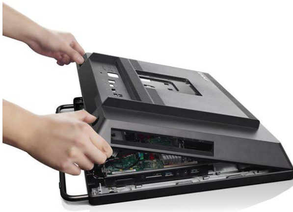
Toolless Back Cover Removal
