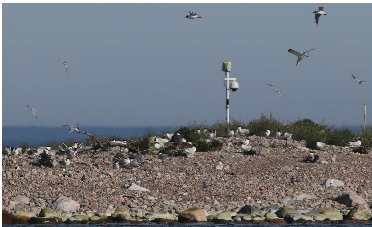
Figure 18. The upgraded webcam camera on Stenarna. This camera can rotate and zoom in on details, for example rings. This has made it possible to read a large number of color rings as well as some metal rings. Reading the metal rings is more difficult as the code on them wraps around the entire ring, meaning that the terns need to cooperate and turn 180 degrees in order for them to be read. Photo by Ulrik Lötberg.
