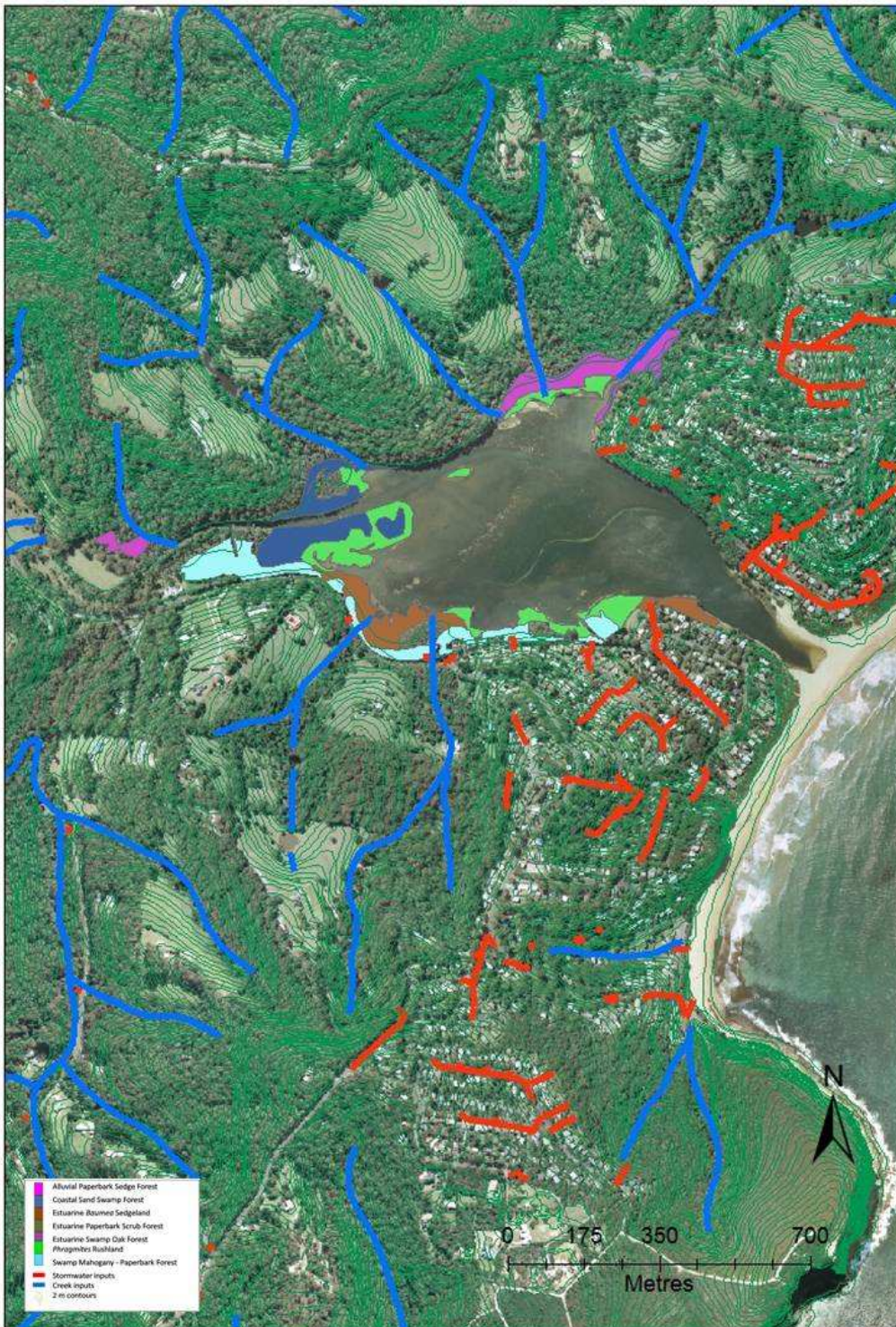
Figure 3.6 Stormwater input map of Cockrone Lagoon showing wetland communities, stormwater pipes (red) streams (blue) and 2 m contour lines (green)
