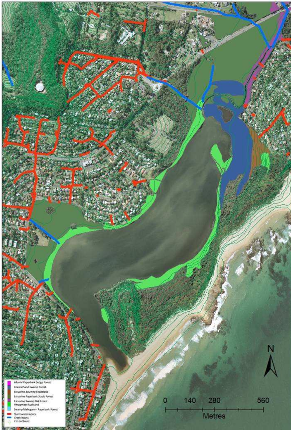
Figure 3.3 Stormwater input map of Wamberal Lagoon showing wetland communities, stormwater pipes (red) streams (blue) and 2 m contour lines (green)
