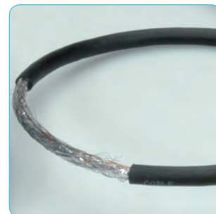
Bad Shielding Cheap Cable
