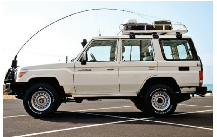
Codan 3040 antennas in horizontal (NVIS) format for short distance (<400KM)
