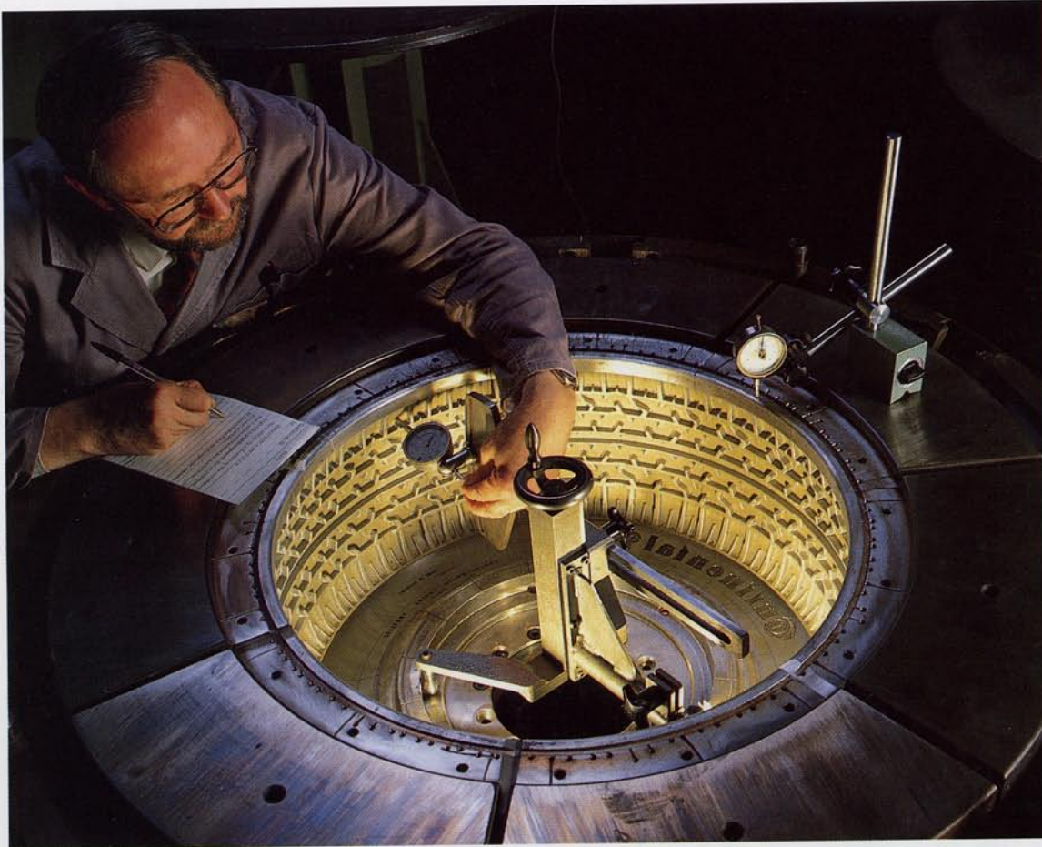
Absolute precision during mold construction is vital to tire uniformity.
