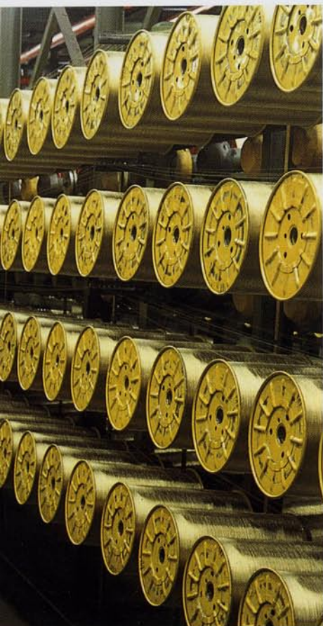
Steel cord is an indispensable reinforcing component of modern radial tires. The wires run from the creel to the calender for rubberizing.
