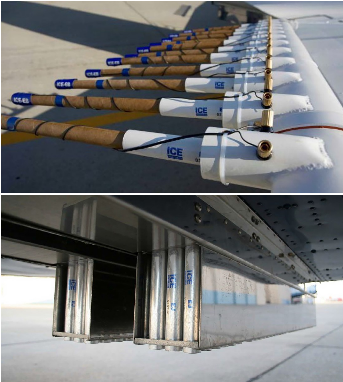
Figure 2-5. Delivery Methods: Wing-Mounted Burn-in-Place Flare Racks Mounted on Specialty Aircraft (top); 20-Gram Ejectable Flares Carried on Cessna 340A (bottom)
