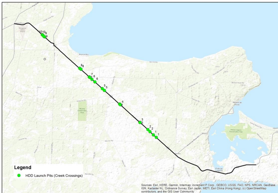
Figure 3. Hydraulic direct drilling (HDD) launch pits
