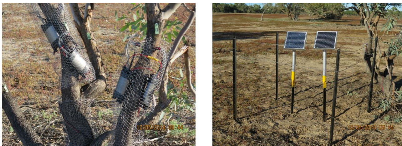
Figure 43 Left, sensors attached to Coolibah trunks. Right, Solar panels powering sensors/loggers
