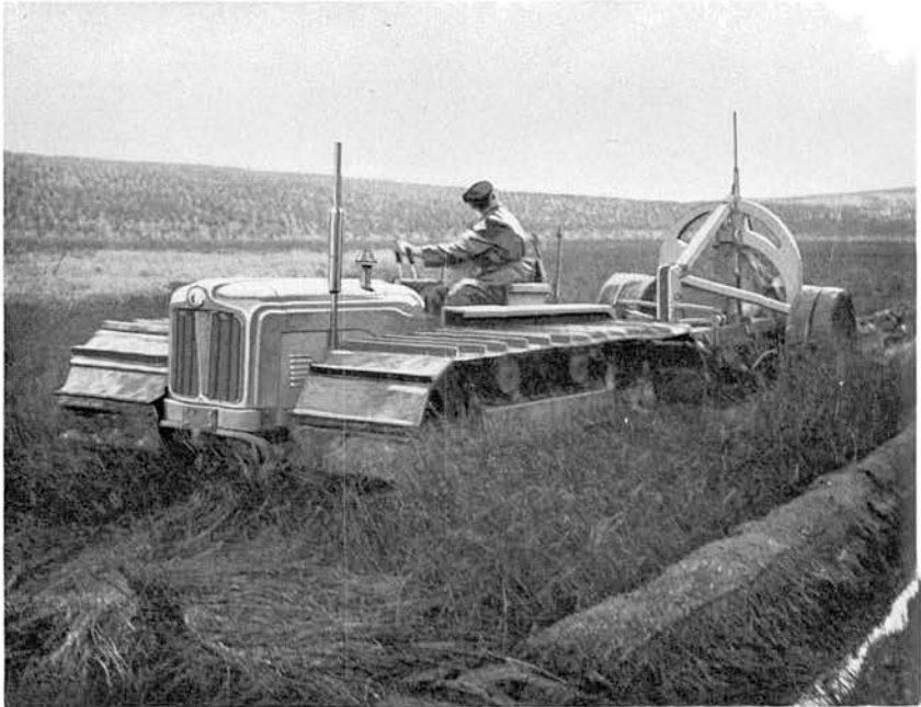
PHOTO 10. Shaw: Machinery Research: Experimental County Tractor with lengthened and widened tracks, drawing a Cuthbertson plough over boggy ground at Kielder Forest, Northumberland.
