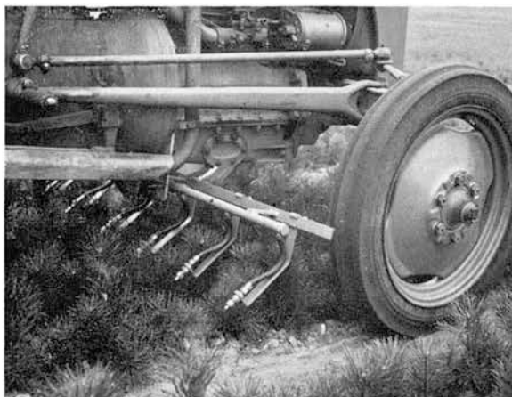
PHOTO 7. Faulkner and Aldhous: Nursery Investigations: Weed Control in Transplant Lines. Tractor-mounted spray boom for applying weedkiller to transplants of Scots pine.
