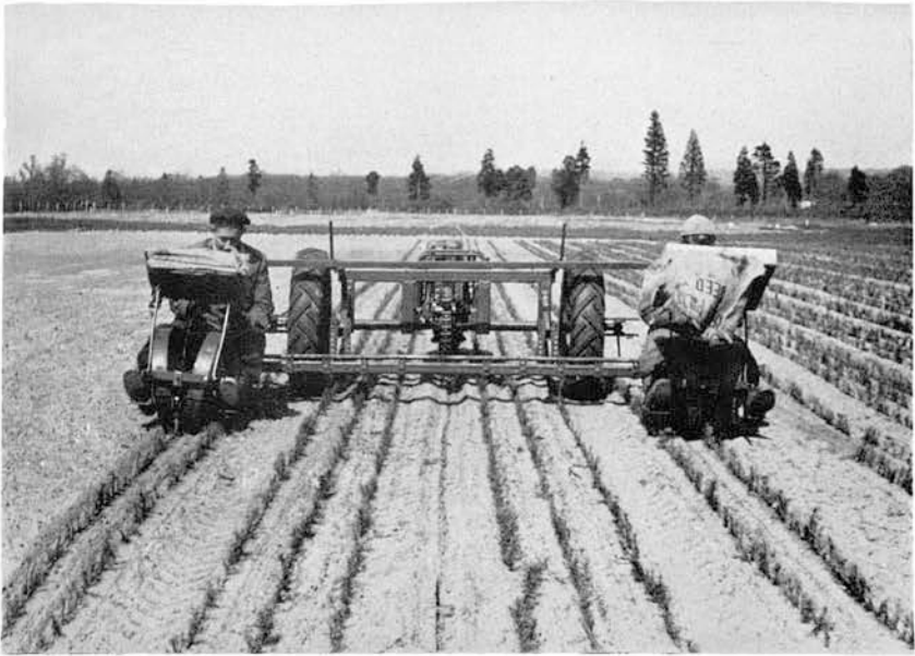
PHOTO 11. Shaw: Machinery Research: Rear view of the Holland Transplanter in operation at Elvetham Nursery, Bramshill Forest, Hampshire. The operators travel backwards, and feed the seedlings into the mechanism.
