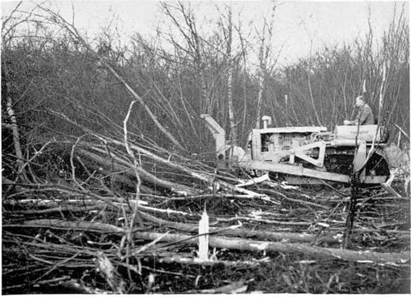
PHOTO 9. Shaw: Machinery Research: Fleco Tree Cutter, mounted on a Caterpillar D4 Tractor, clearing scrub at Waterperry Wood, Bernwood Forest, Oxfordshire.
