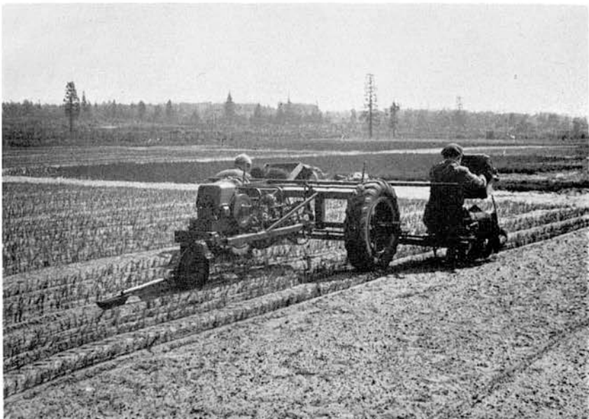
PHOTO 12. Shaw: Machinery Research: Front view of the Holland Transplanter, showing the automatic steering device running in a central groove.
