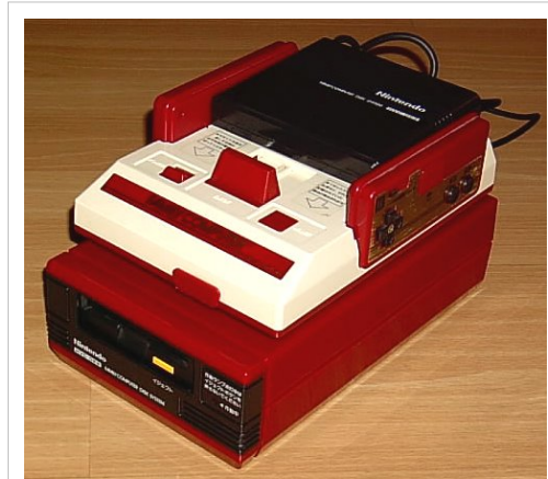
The Famicom Disk System was a peripheral available only for the Japanese Famicom that used games stored on "Disk Cards", reminiscent of 3" Quick Diskettes.
