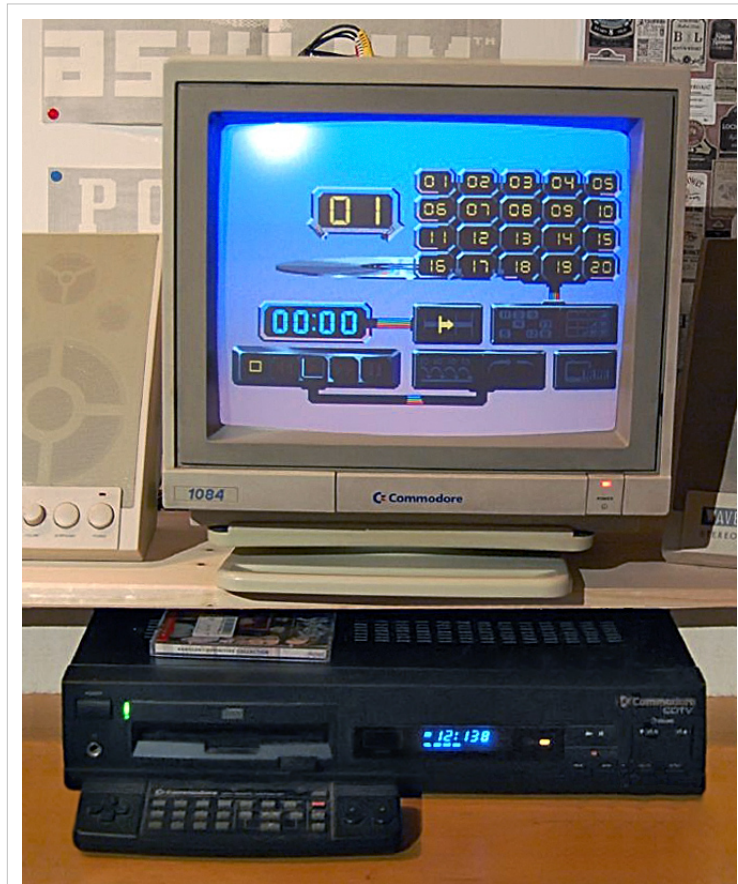
Commodore CDTV setup with 1084 monitor displaying the CDTV's audio CD player facility.
