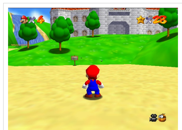
Screenshot of Super Mario 64 , showing limited texture detail and Gouraud shading (on Mario). The trees are two-dimensional billboards and always face the camera.
