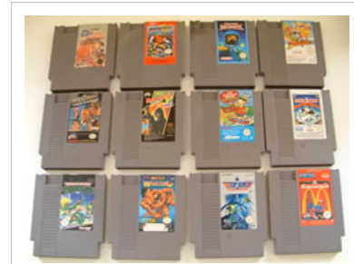
North American cartridges (or "Game Paks", pictured) were significantly longer than their Japanese counterparts, but were not as wide.
