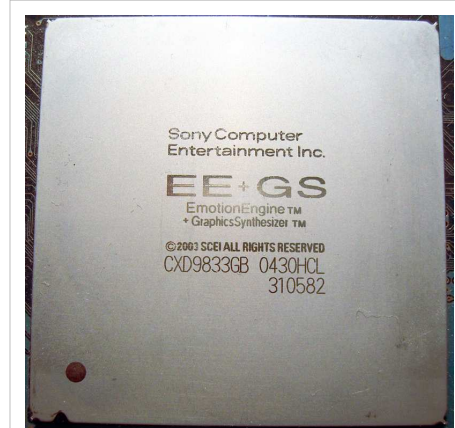
Older EE+GS that does not incorporate system memory (Found in Older Charcoal Black Slim PS2s. (SCPH-70001).
