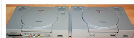
Comparison of the rear of an original SCPH-100x model and a SCPH-900x model. The SCPH-900x revision saw the removal of the Parallel I/O port while the RCA jacks were removed in the SCPH-500x revision.
