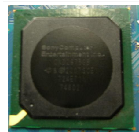
ASIC that incorporates the EE, GS, and system memory (found in silver slim PS2s. Model SCPH-7900x and later).
