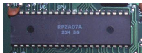
Versions of the NES console released in PAL regions incorporated a Ricoh 2A07 CPU.
