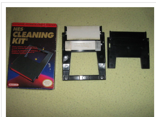
The official NES Cleaning Kit was intended to address flaws in the NES design that caused cartridge connectors to be particularly susceptible to interference from dirt and dust.
