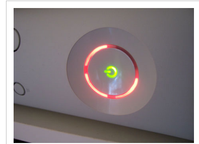
The Xbox 360 displaying three red lights, indicating a "general hardware failure" (often referred to as a "red ring of death")
