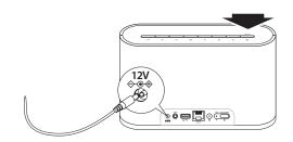
press & hold **(b)** power button (3 seconds) to power ON iW2
