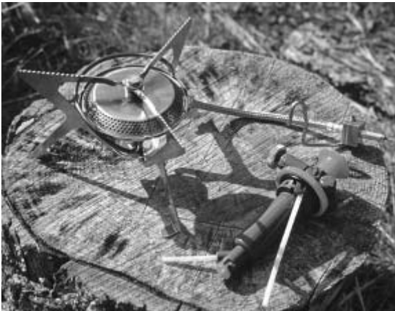
TOP: The MSR DragonFly multifuel stove offers separate flame control, which is good for simmering. ABOVE: The MSR SimmerLite white-gas stove is the lightest white-gas stove available.
