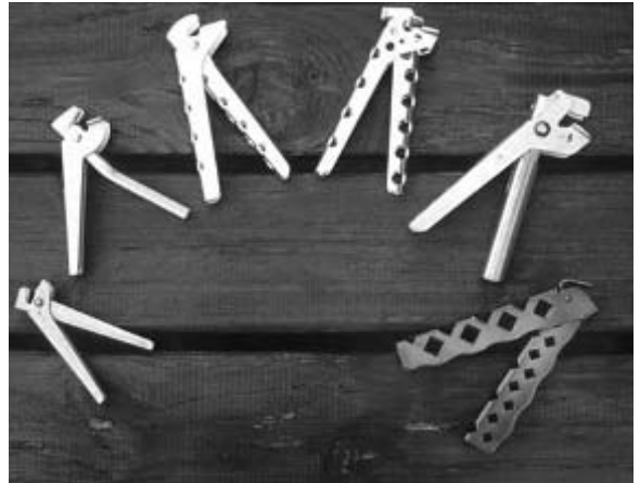
A selection of pot grippers for pots of different sizes. You'll need the larger ones for pots that hold more than a quart.
