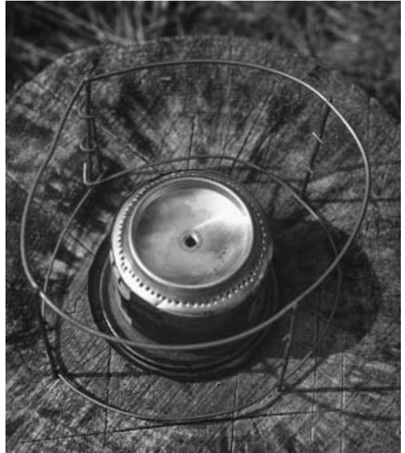
Homemade soda-can alcohol stove with wire pot support, made by Jake Schas. While inexpensive and very light, this stove lacks any flame control.
