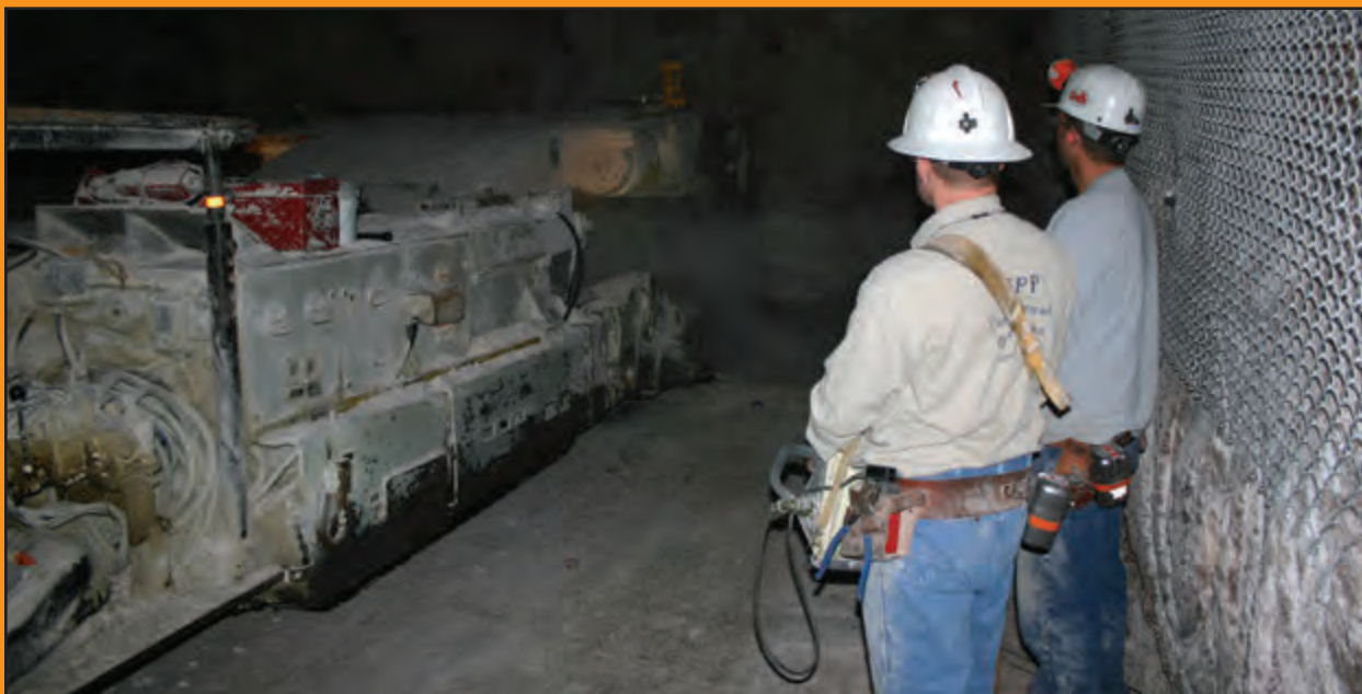
Miners use a remote-controlled, continuous-mining machine to make space in the bedded salt for planned salt disposal investigations at the Waste Isolation Pilot Plant, 2011.
