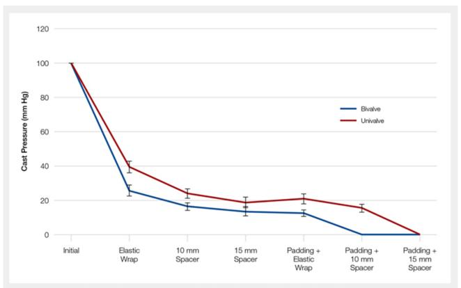
Figure 5. Graphic representation of pressure measurements at each study time point according to cast type (univalve or bivalve).
