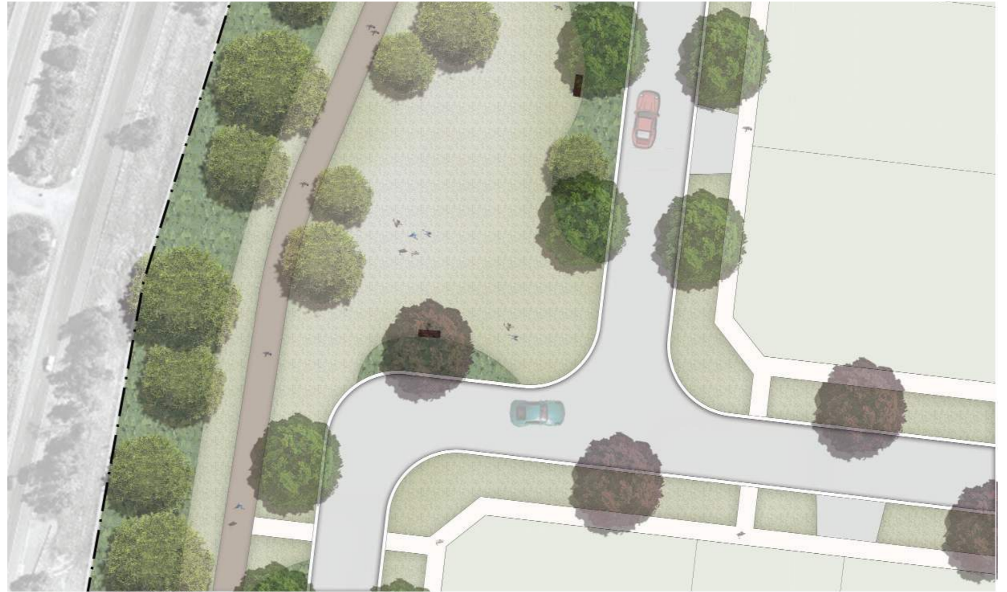
Plan of typical 16m access street - adjacent to freeway acoustic fence & reserve
