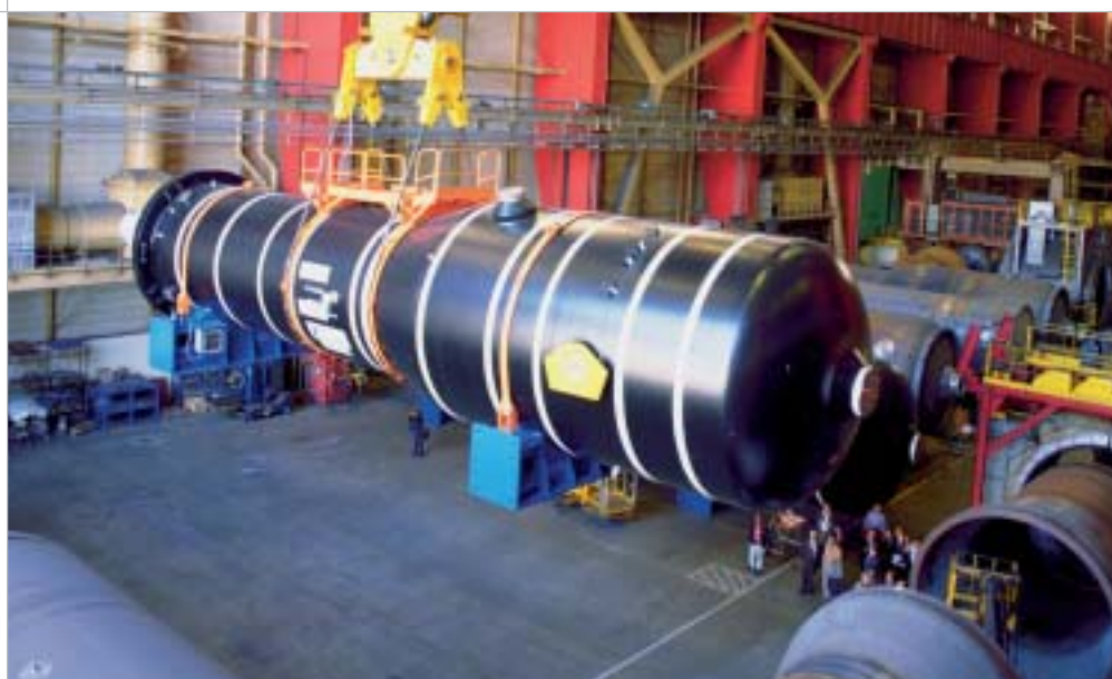
900MW steam generator, FRAMATOME ANP plant (Chalon-Saint-Marcel, France)
