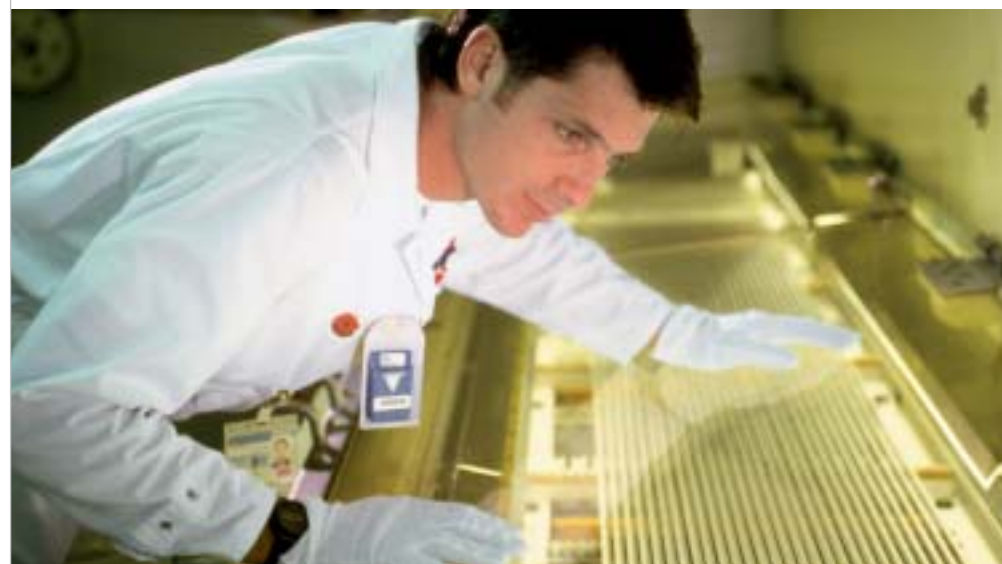
MOX pellets are loaded into metal fuel rods used to make MOX fuel assemblies.
