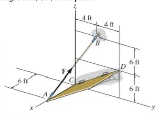
Moment About the CD axis: Either position vector  $\mathbf{r}_{CA}$  or  $\mathbf{r}_{DB}$ , Fig. a, can be used to determine the moment of F about the CD axis.
