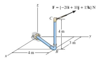
Moment About Line AB: Either position vector  $\mathbf{r}_{AC}$  or  $\mathbf{r}_{BC}$  can be conveniently to determine the moment of F about line AB.
