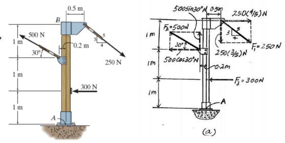
Equivalent Resultant Force: Forces  $F_1$  and  $F_2$  are resolved into their x and y components, Fig. a. Summing these force components algebraically along the x and y axes,
