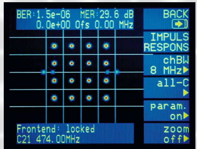
FIG 9 Constellation diagram in the R&S®EFL 100; the frequency distribution of the individual symbols is marked in color.
