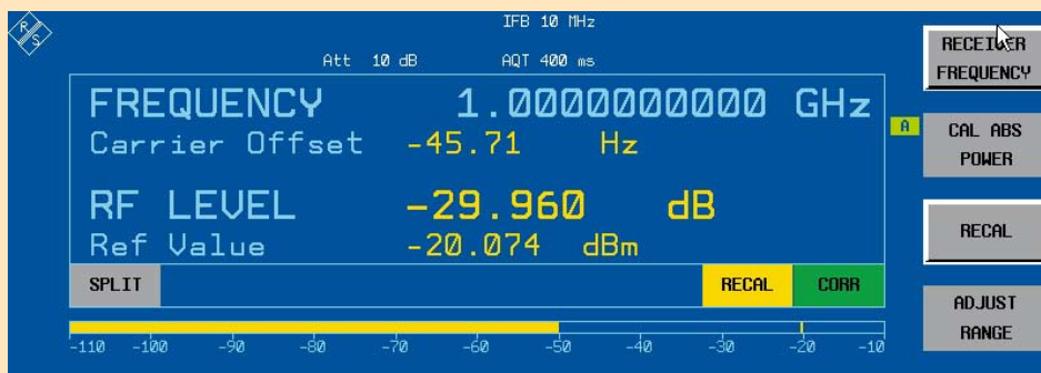
FIG 2c If the level is changed and the measurement range limits have been reached, the R&S®FSMR activates the yellow RECAL field to inform you that you need to calibrate the adjacent range.
