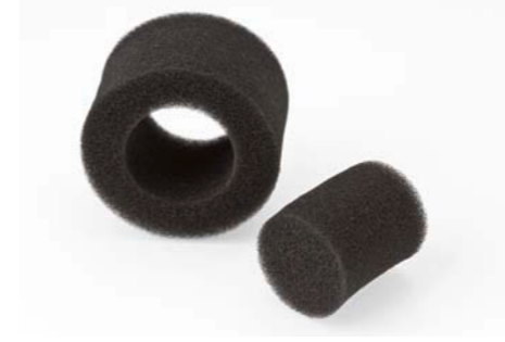
Vario Bass Control (VBC, Vario BC) Two-part plug to influence bass level. Reduces the effective cross-section of the bass reflex tubes in two stages. For bass reflex tube with 70 and 55 mm diameter.
