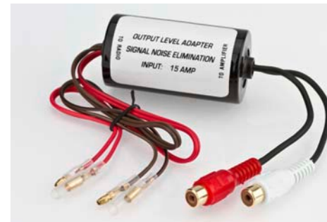
High-low line level converter High-low line level converter. Problem solver for sources which have only one loudspeaker output (no line output) (e.g. mini- or midi-systems) to connect active loudspeakers to such sources. Galvanic decoupling of input and output signal by transformers, with level conversions of loudspeaker level to line level.
