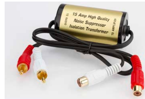
Ground loop isolator Ground loop insulator. Problem solver when it comes to hum pickups (e.g. with some notebooks near active loudspeakers) for galvanic decoupling of input and output signal by transformers. Without level loss. For direct looping into an existing RCA connection.
