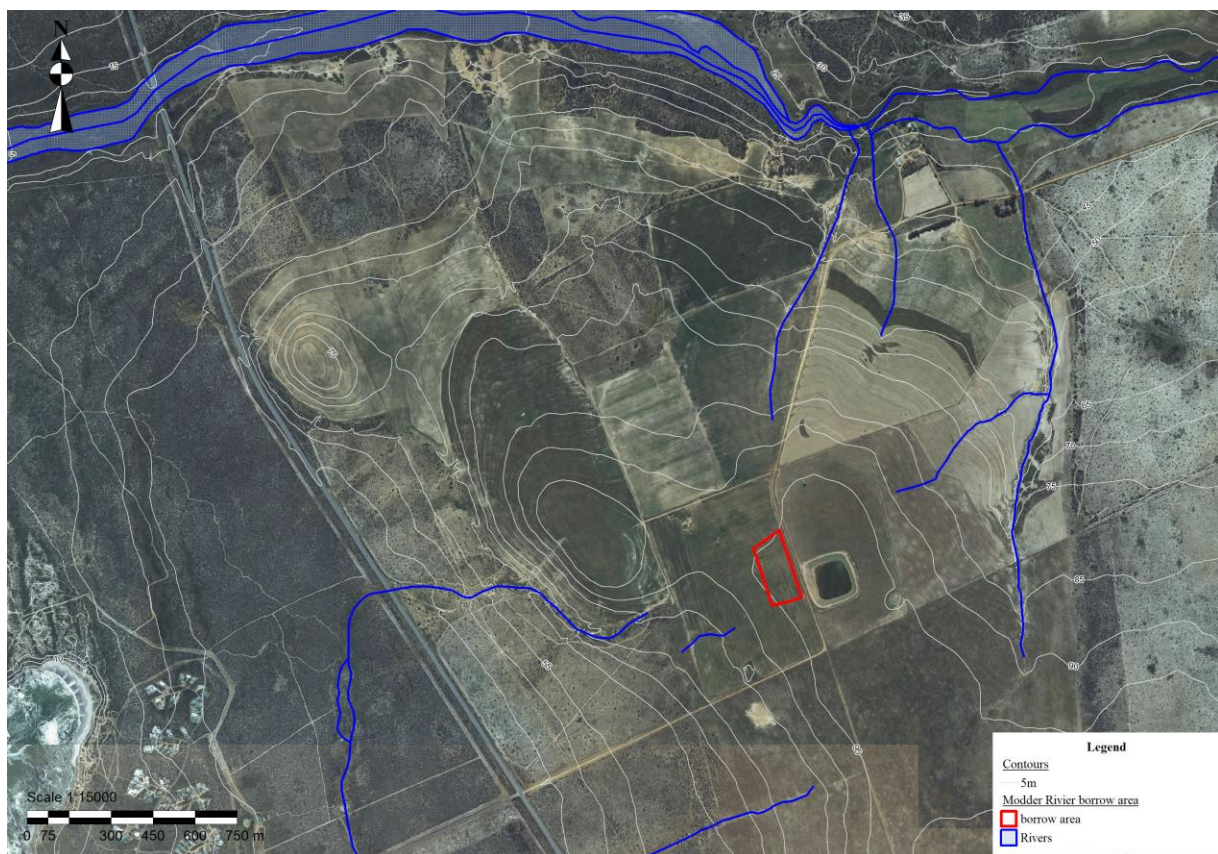
Figure 2. Orthophotograph of the proposed borrow pit area and surrounding area with the watercourses indicated as well as the 5m contours
