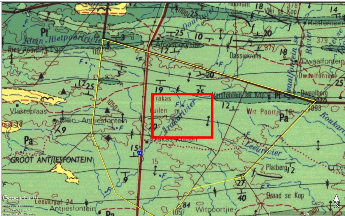
Figure 6-22: Extract from 1: 250 000 geology sheet 3222 Beaufort West (Council for Geoscience, Pretoria) showing geology of combined Beaufort West Cluster wind farm project area situated either side of the N12 national road (yellow polygon) as well as the approximate location of the present study area for on-site substation and associated infrastructure 26 .
