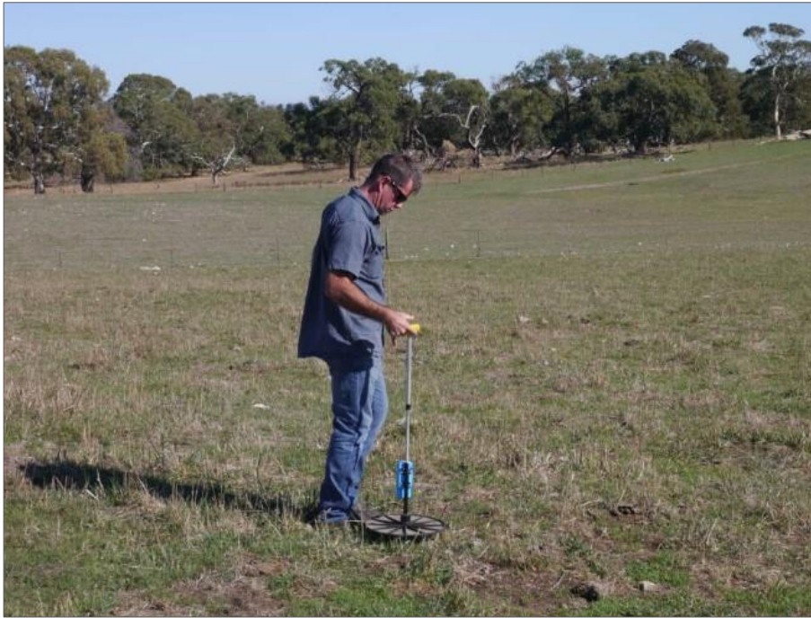
Figure 7.2: Farmer operating a disc pasture meter to estimate standing biomass (Photo: Amber Wood).
