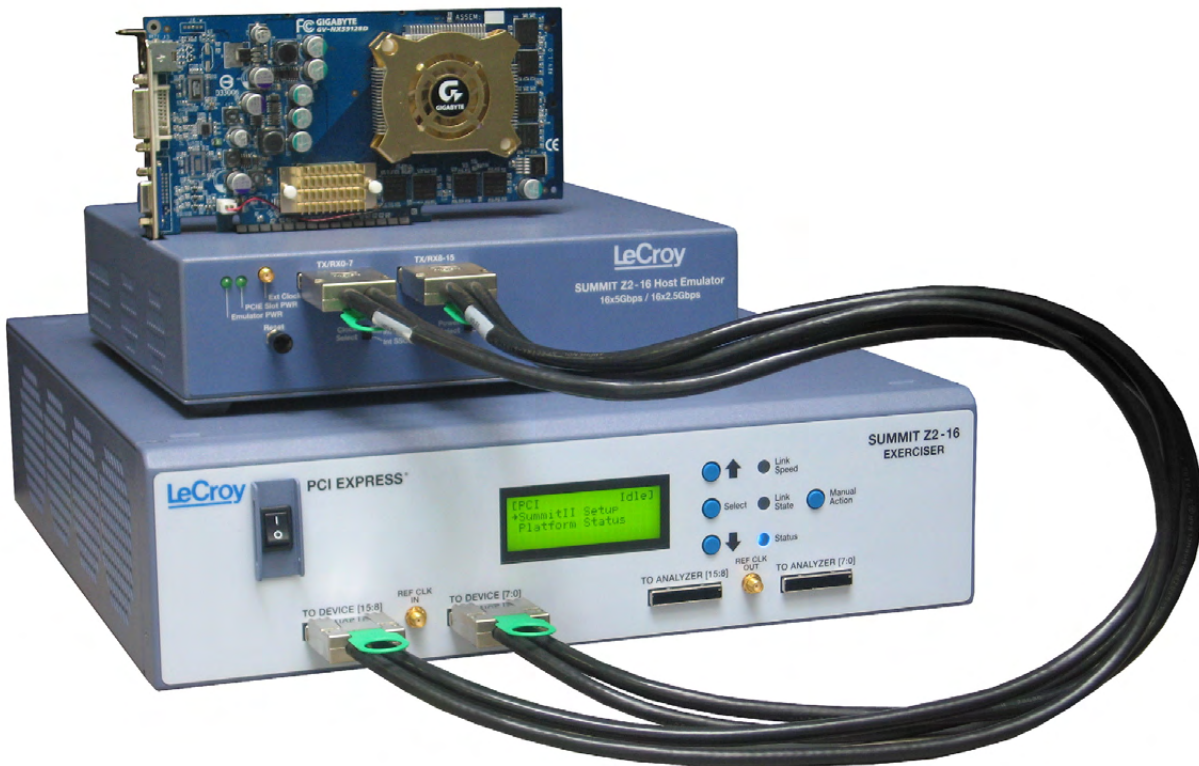
Figure 3.4 Summit Z2-16 Exerciser (bottom) connected to a Host Emulator adapter (top). The Host Emulator has a PCI Express graphics card inserted.
