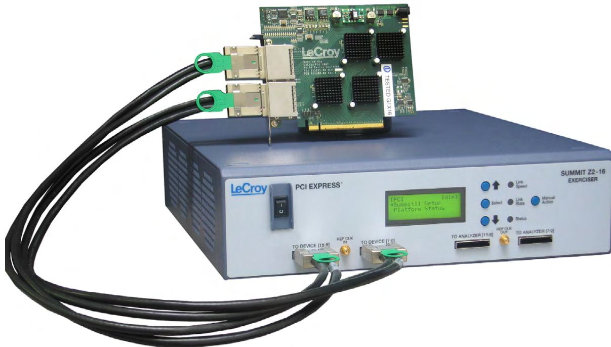
Figure 3.3 Summit Z2-16 Exerciser (bottom) connected to a Device Emulator (top).
