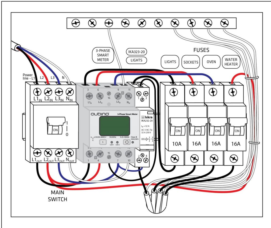
**For controlling electrical devices with IKA232-20/230V and one with BICOM432-40-WM1:**
