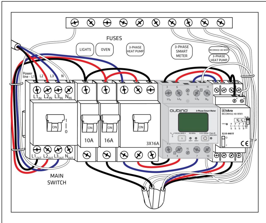
**For controlling one electrical device with IKA232-20/230V:**
