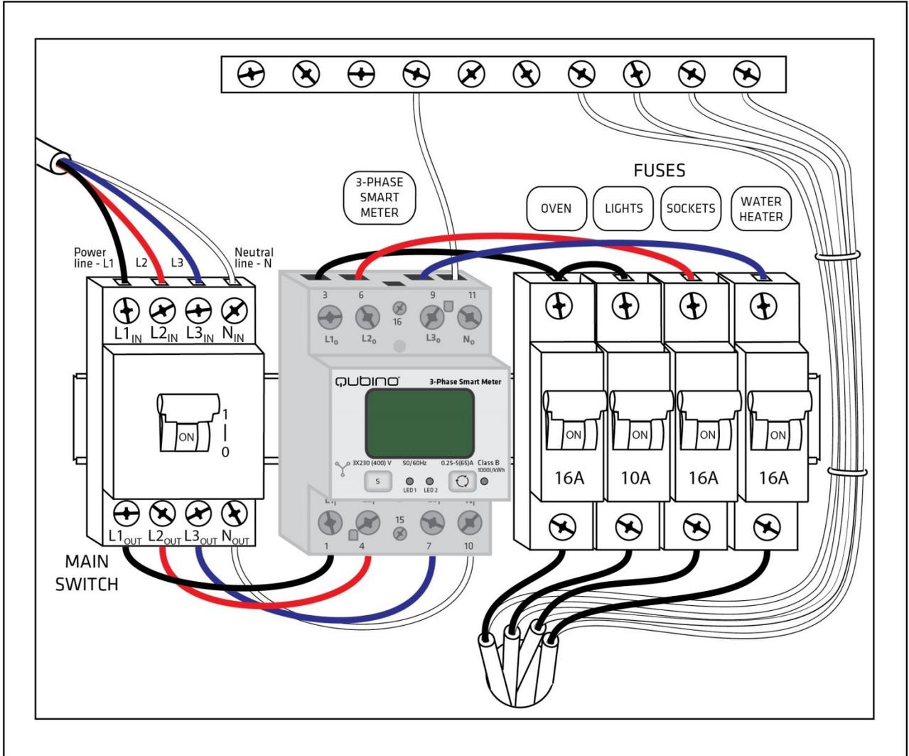
**For controlling one electrical device with BICOM432-40-WM1\*:**
