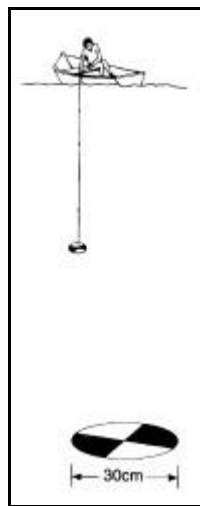
Figure 2.4 The use of a secchi disc to assess vertical water clarity. The secchi disc is lowered into the water until the black and white quarters are no longer distinguishable. The length of rope from the surveyor to the disc is then recorded (m). Source: English et al. (1997).
