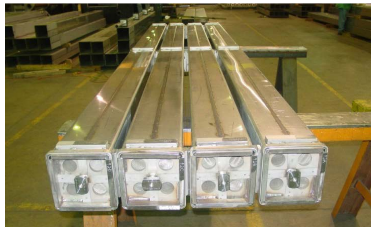
Damaged Fuel and Waste Containers (made from stainless or neutron absorber) over 100 loaded and 44,000 on order for CHNPP
