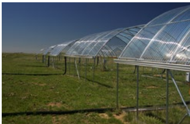
Extreme Drought in Grasslands (EDGE) rainfall reduction shelters in the semi-arid shortgrass steppe grasslands of Colorado (USA). Photo: A. Knapp.
