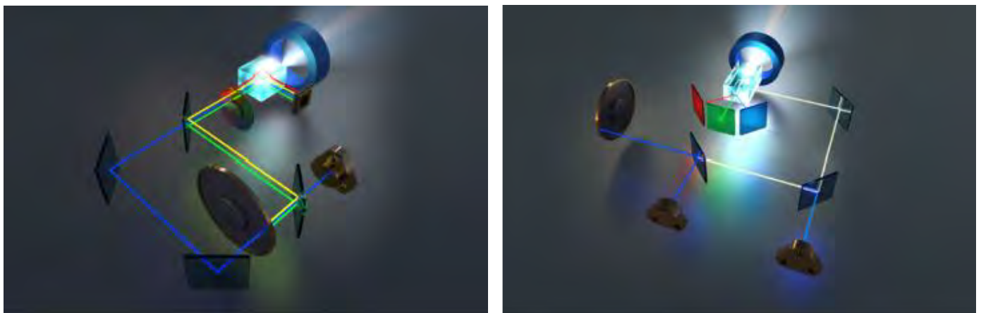
Figure 2 & 3 – Laser Phosphor Light Path for 1x DLP (left) & 3x DLP (right)
