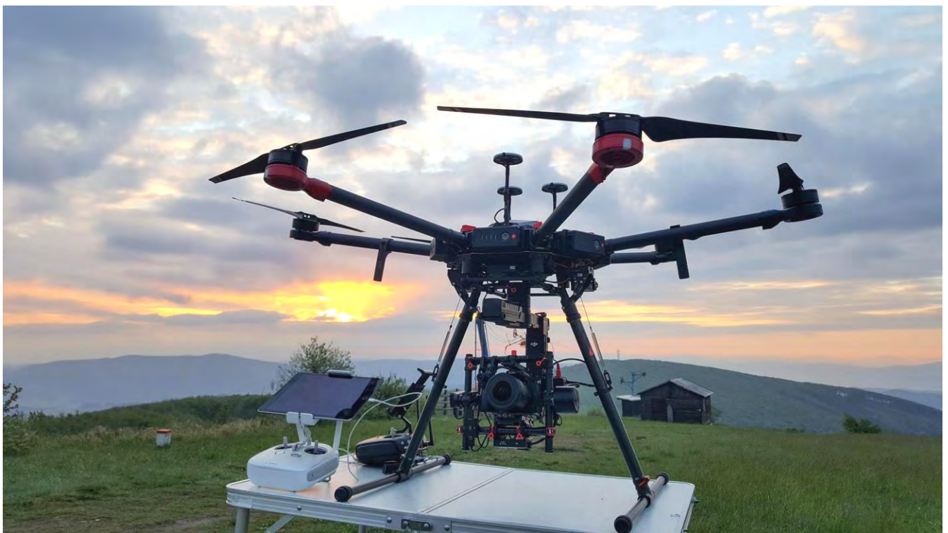
Figure 1 – DJI Matrice 600, Panasonic GH4 and Sigma 4.5mm f/2.8 fisheye (photo courtesy: UpVision)
