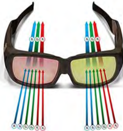
Figure 7 – Separation of light of a 6P source in 3D application (courtesy of Christie Digital Systems Inc.)
