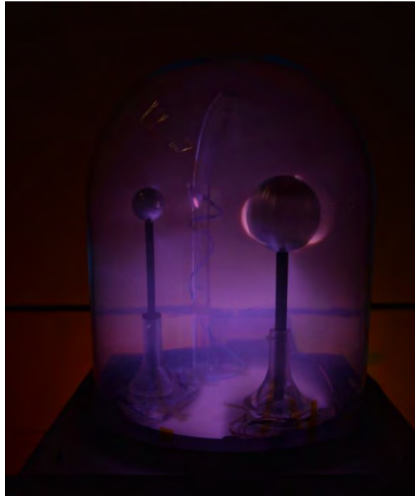
Figure 8 – Planeterella in action with the overall present light purple glow, this is the representation of the Sun's corona.
