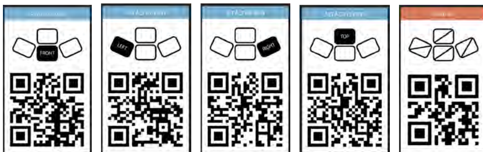
Figure 1 – QR codes for operations which can be incorporated into a presentation and detected by our display software. The graph in the upper section indicates what kind of operation the presenter wants to achieve.
