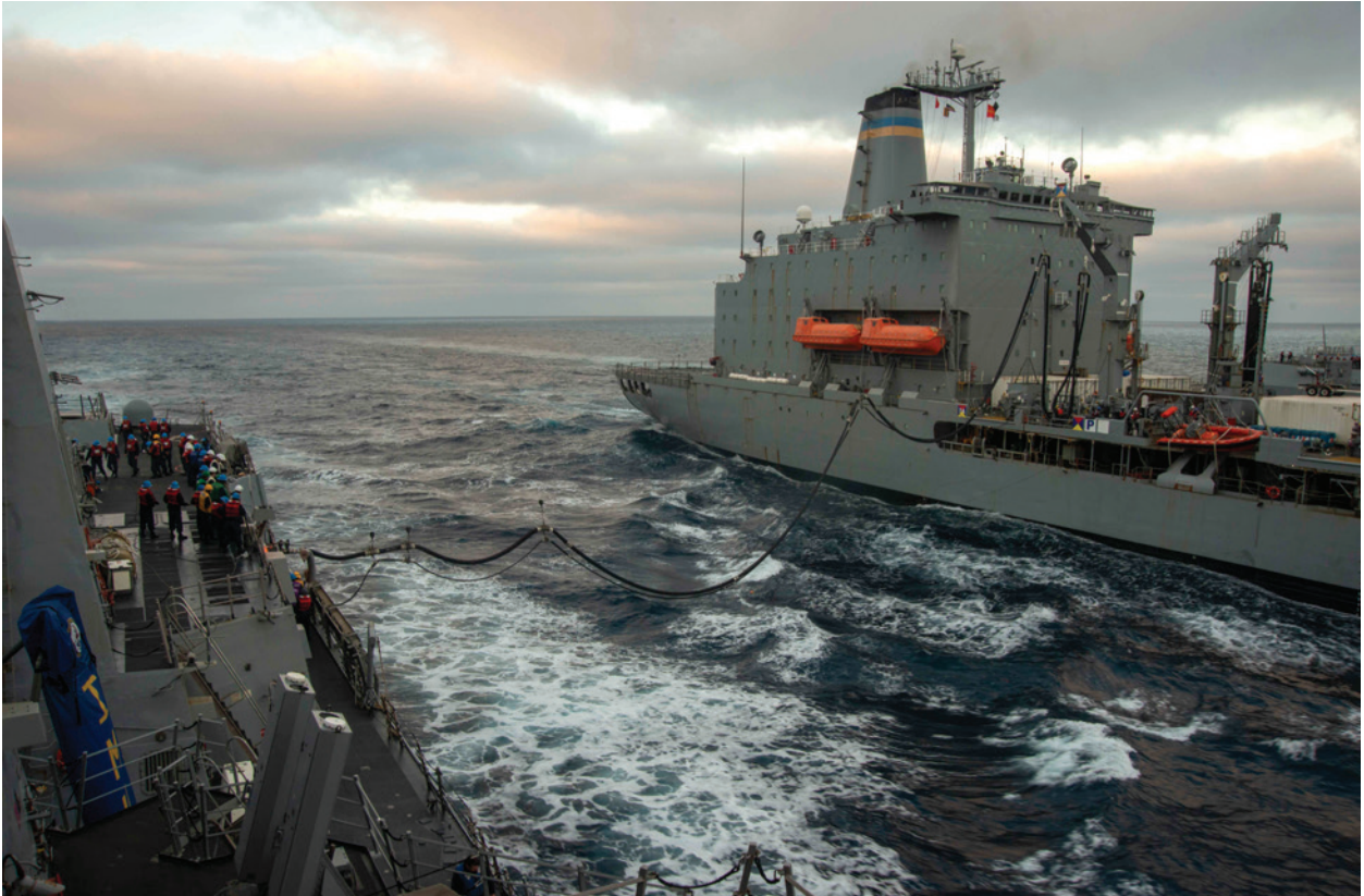
PACIFIC OCEAN (Oct. 9, 2022) The Arleigh Burke-class guided-missile destroyer USS Chung-Hoon (DDG 93) takes on fuel during a replenishment-at-sea with the fleet replenishment oiler USNS Henry J. Kaiser (T-AO 187). Chung-Hoon is currently operating with Nimitz Carrier Strike Group in preparation for an upcoming deployment. (U.S. Navy photo by Mass Communication Specialist 3rd Class Kenneth Lagadi)
